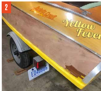
A corner of the previous repair was already coming off due to poor adhesion. FIG. 2
