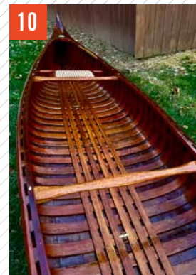
The entire floor rack was coated with 105/207 and topped with varnish. FIG. 10
