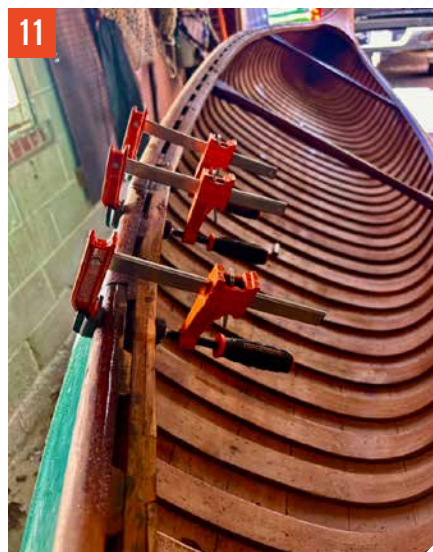
New pieces had to be scarfed into the gunwales to fill missing sections. FIG. 11
