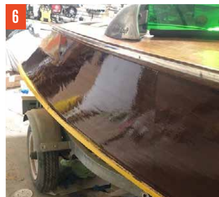
105 Epoxy Resin and 207 Special Clear Hardener were applied over the new wood veneer. FIG. 6
