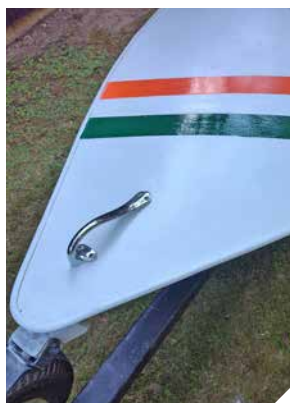
Faired and painted, with the handle reinstalled.
