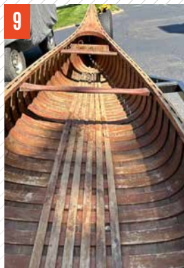
The removable floor racks were so rotted that they had to be completely rebuilt from white oak. FIG. 9
