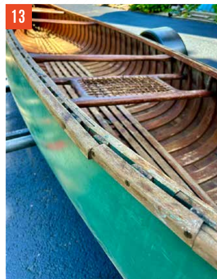
There were a couple of damaged sections along the gunwale. FIG. 13
