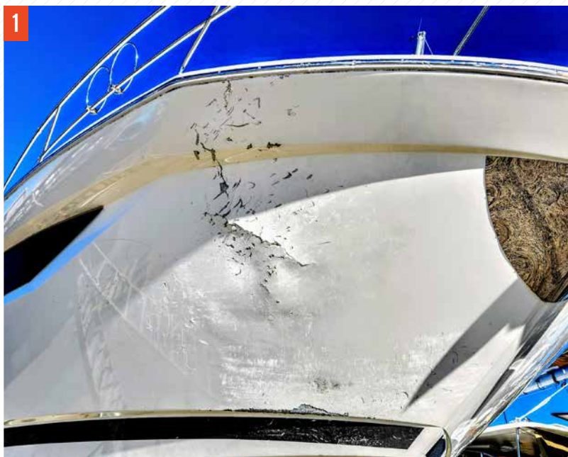
The damaged fiberglass once the boat was hauled out. FIG. 1
