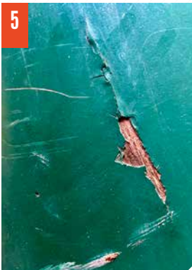
A couple of gouges damaged the skin of the canoe. The gaps were filled with Six10. FIG. 5 & 6
