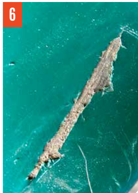
A couple of gouges damaged the skin of the canoe. The gaps were filled with Six10. FIG. 5 & 6
