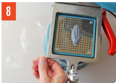
8 Remove the molded plastic. Let the pattern cool down before repeating the cycle.
