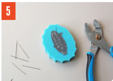
5 Let the epoxy cure overnight and then remove the pins.
