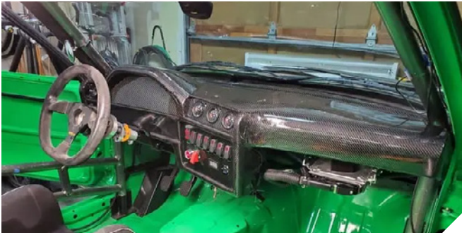
Example of carbon fiber skinning previously featured in Epoxyworks.
