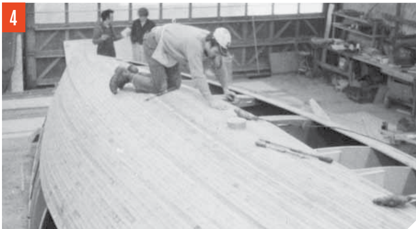
STRIP PLANKING Narrow strips are edge glued over a frame. Though popular on canoes and kayaks, this strip planking is on a 42' (12.8 m) hull.
