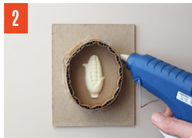
2 Hot glue a strip of cardboard around the model.
