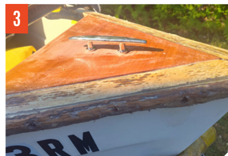
Bow piece installed. The damaged gunnel needs to be replaced.
