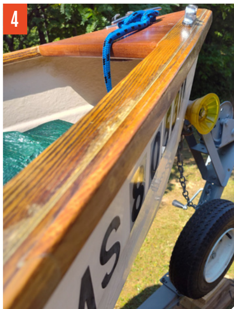
Looking down the length of the replaced gunnel section.
