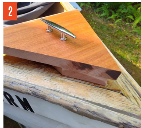
Fitting the replacement bow piece.
