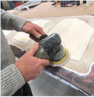
Orbital sander was used to create the final profile and flattened bevel angle.
