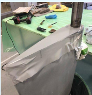
Surface is coat with tinted epoxy to seal top surface of rudder.
