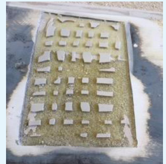
The router is moved over the epoxy to remove a majority of the epoxy to maintain 0.125" depth.
