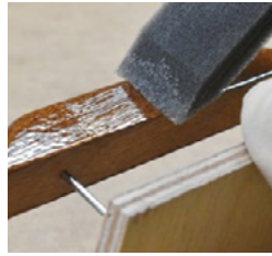
Rolling with 800 Roller Cover and tipping with foam brush.
