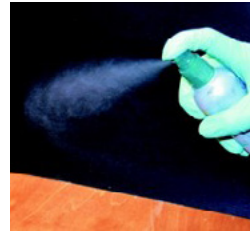
Misting with Denatured Alcohol to remove air bubbles.
