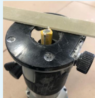
1/8" thick G-10 is used as a guide to set router depth.
