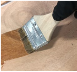
Bristle can be cut shorter to increase stiffness for application.
