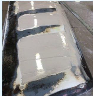
Surface of the rudder is faired with epoxy.
