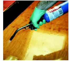
Using a propane torch to remove air bubbles.
