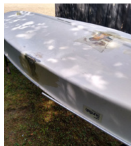
Previous patch attempts were rough. They needed to be reinforced and ground fair with the hull.
