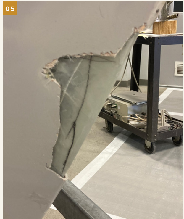
Foam mold removed. Test fitting backer plate.
