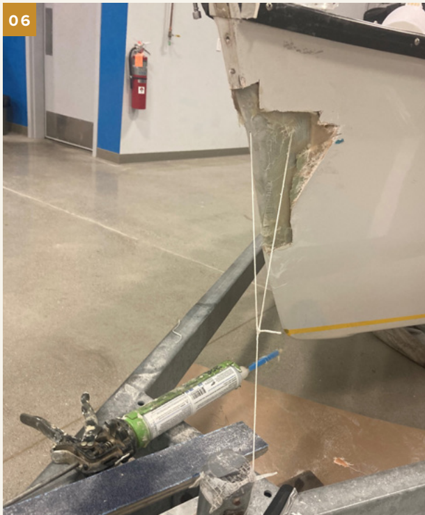
Six10 Thickened Epoxy Adhesive was used to bond the backer to the hull.
