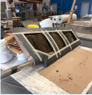
All wet foam is removed from the inside of rudder.
