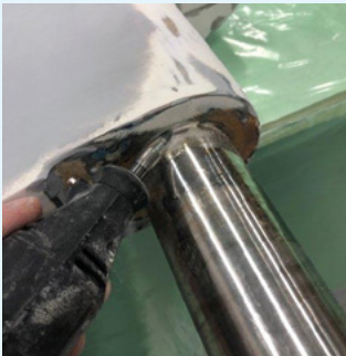
Rotary tool used to increase surface area around top shaft of rudder.
