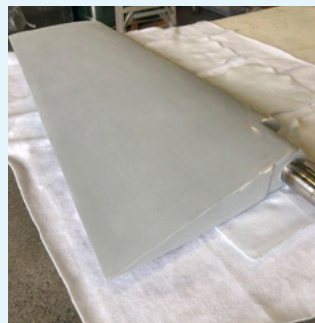
Rudder ready for application of paint.
