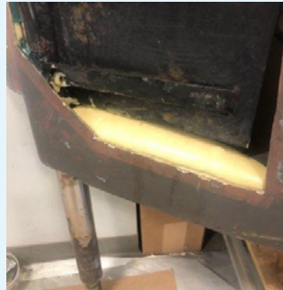
Foam is poured into top of rudder.
