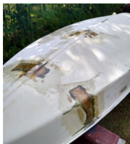
Previous patch attempts were rough. They needed to be reinforced and ground fair with the hull.
