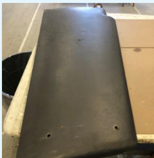
Rudder with a few drilled holes to check the foam's integrity.
