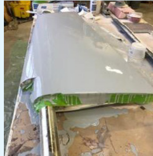
Tinted epoxy over entire surface of rudder.
