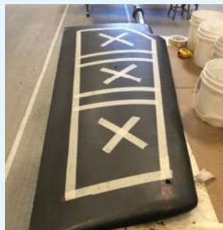
Masking tape used to mark the area that would be cut away.
