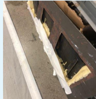
Rudder is laid on its side and leading edge is filled with foam.
