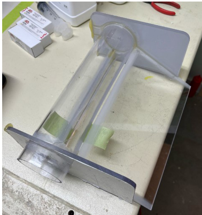
Planer chip diverter, custom built from polycarbonate and G/flex epoxy.
