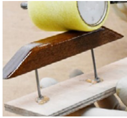
Rolling with 800 Roller Cover and tipping with foam brush.
