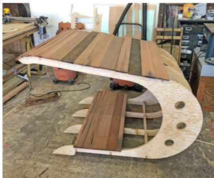
The ribs were cut from marine fir plywood, and the cladding was salvaged redwood planks.
