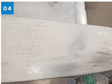
04 The high areas have been sanded down into old fairing compound and fiberglass. The remaining pencil lines indicate the low areas where the new fairing compound needs to be applied.
