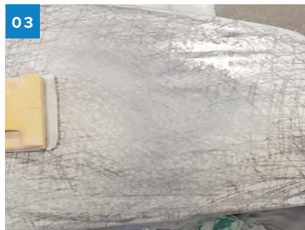
03 Sand pencil marks to reveal high and low areas.
