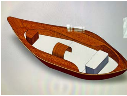
CAD rendering of the drift boat design prior to start of build.
