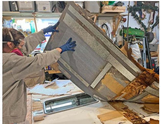
Peeling back the luan panel seeing the true extent of the water damage.
