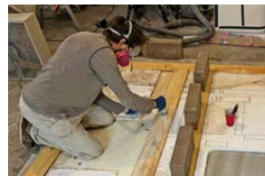
Applying a neat coat of epoxy before bonding the plywood to the fiberglass wall panel.
