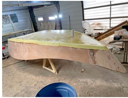
The boat after primary hull construction. Note the rounded transom on the right, recurve sides, and Kevlar fabric on the bottom and chines.
