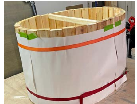
Ratchet straps were used to draw the vertical strakes together while the epoxy cured.
