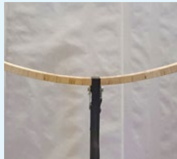
The pine repair broke where the balsa core met the pine.
