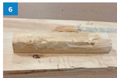
Pine still glued horizontally on plywood with epoxy after removal attempt.
