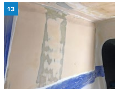
13 80-grit was used to sand away the paint on the daggerboard case.
