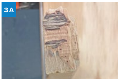
The broken or "failed" surface of the plywood glued with yellow glue.
