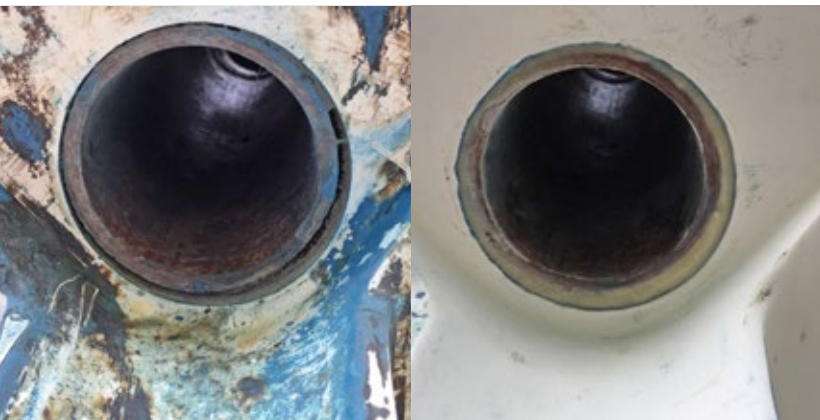
TOP: The rudder shaft before and after repair.
