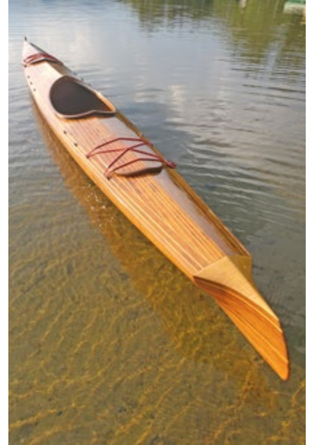
Kevin Triplett of Boston, Massachusetts designed and built this kayak using WEST SYSTEM 105 Resin, 207 Special Clear Hardener, and 403 Microfiber Filler.
