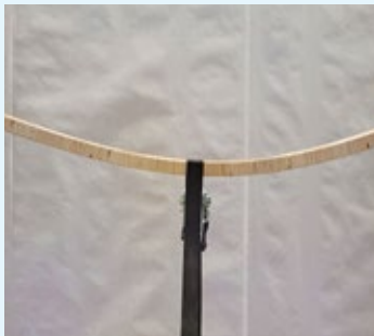
The balsa cored control sample cracked in half when it broke.
