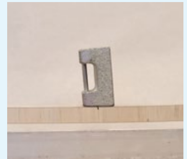
The end grain pine repair was only a little stiffer.
