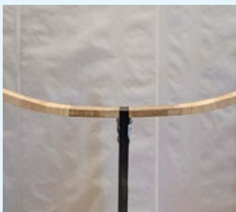
The plywood repair broke where the balsa and plywood met.
