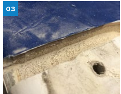
03 A router was the best tool for removing the high-density foam core.
