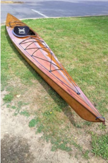
Alan Bergen built this Bear Mountain resolute kayak using 6 oz glass on the hull, 4 oz glass on the deck, WEST SYSTEM 105 Resin® and 207 Special Clear Hardener®. The trim is walnut and pine.
