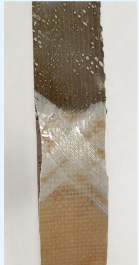
The fiberglass fractured in compression at the transition from epoxy to balsa core in the epoxy-filled repair.
