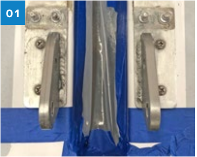
01 The aluminum mounting brackets on the mast step.
