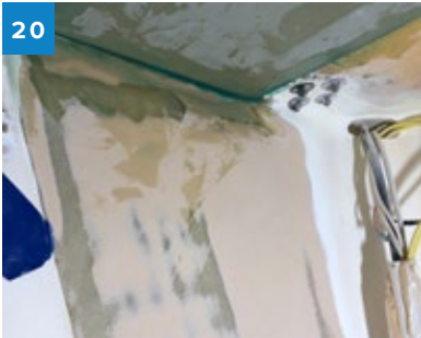
The port side G-10 panel was bonded underneath the deck with Six10.
