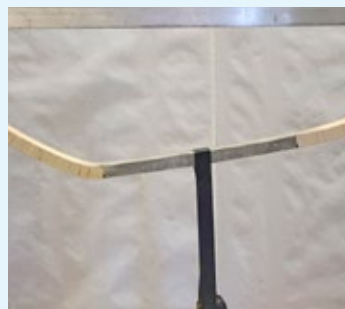
The epoxy filled repair broke most dramatically, again at the repair joint.
