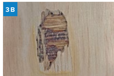
The broken or "failed" surface of the plywood glued with yellow glue.
