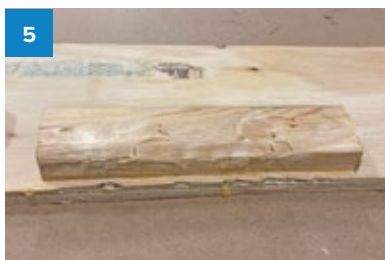
Pine still glued horizontally on plywood with yellow glue after removal attempt.
