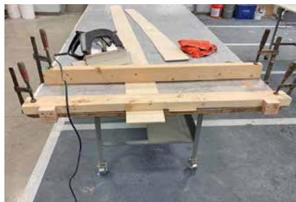
The fence clamped to the plywood with additional secondary clamped 2"x4".
