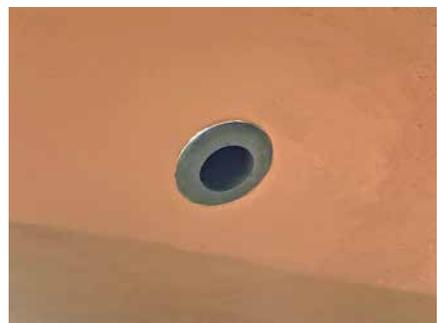
Left: We tapered the unneeded hole at a 12:1 bevel. Middle: New fiberglass patches are applied to the hull. Right: The final thru-hull after applying anti-fouling bottom paint.
