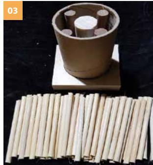
03 Epoxy the four darker colored dowels to the base inside the mailing tube, around the center dowel.
