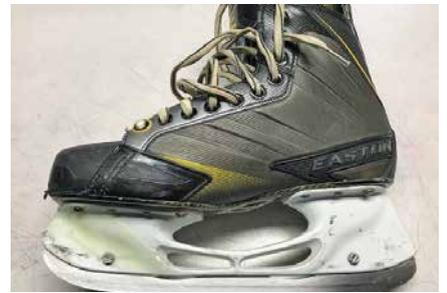
Chet Asher of Ocean City, New Jersey repaired the broken blade holder on his hockey skate with 105 Resin/205 Fast Hardener and 6 oz. fiberglass cloth.
