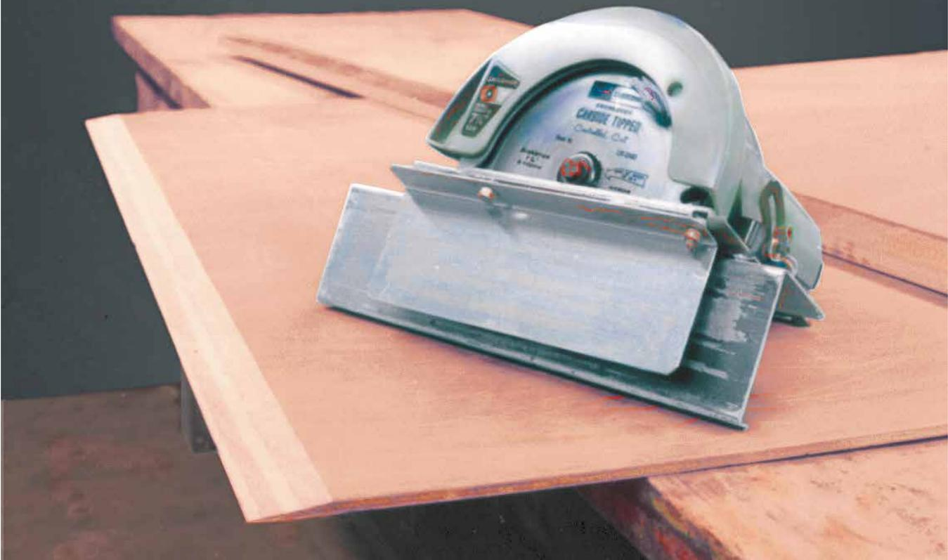
Scarfig wood together dates back ages. Scarfig is the process of cutting corresponding angles (or sometimes shapes) on two similar pieces of wood and gluing them together to create a larger piece of lumber or plywood. The most common place scarfig is used is in building a stitch-and-glue canoe or kayak.
