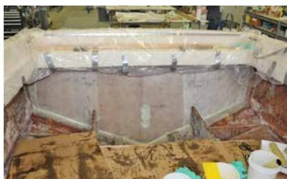
*Fiberglass has been applied to the transom and tabbed on to the hull.*
