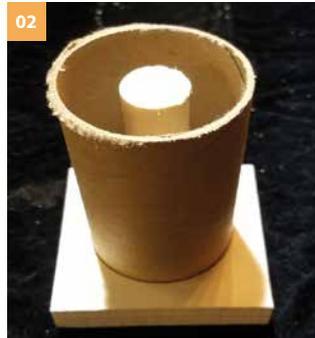
02 Epoxy the 3/4" dowel to the base, at the center of the mailing tube.
