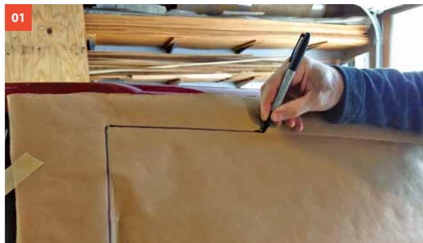
1. Create a template using clear plastic film or craft paper on the car window opening. Make the template large enough to cover a half-opened side window.
