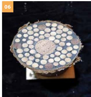
06 Slowly pour the epoxy mixture into tube and allow it to cure.
