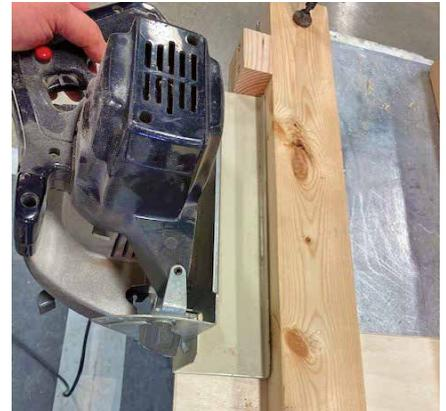
Cutting the scarf at an 8-to-1 bevel.
