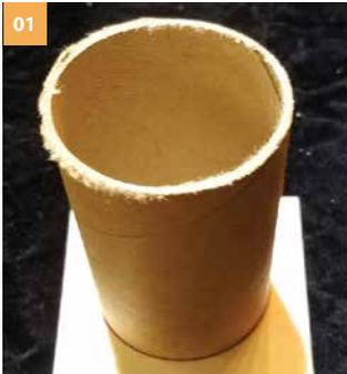
01 Mix a small batch of 105/207 epoxy and adhere the mailing tube to the base, allow to cure.
