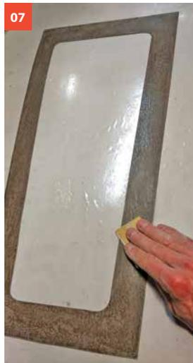
7. Allow the epoxy to fully cure, then sand surfaces dull and remove any burrs from the edges.
