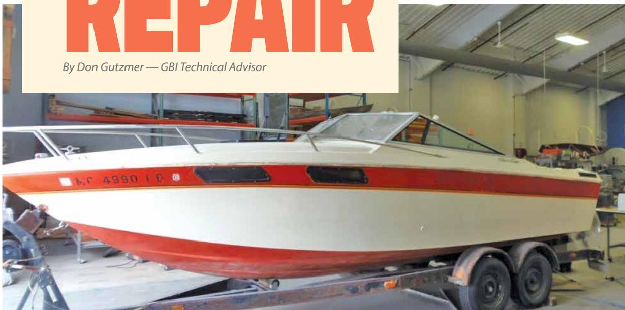
In order to demonstrate proper repair methods, our Technical Department purchased a neglected 1980 Chris Craft Scorpion 230 in need of a complete restoration. It had rotted stringers, transom, cockpit sole, and other problems common in fiberglass boats. I'll explain the process we used for replacing the transom to provide some direction on tackling similar projects.
