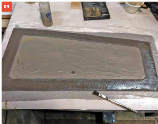
9. Flip the screen frame over, dull the backside with sandpaper, and glue in plastic window screen fabric (available at hardware or building supply stores) with G/5 Five-Minute Epoxy. Allow the epoxy to cure.
