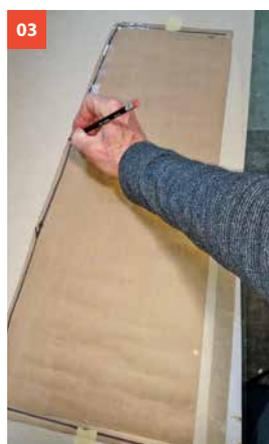
3. Transfer the template to your cardboard or fiberglass screen frame stock. Cut to shape with scissors, snips or a utility knife.
