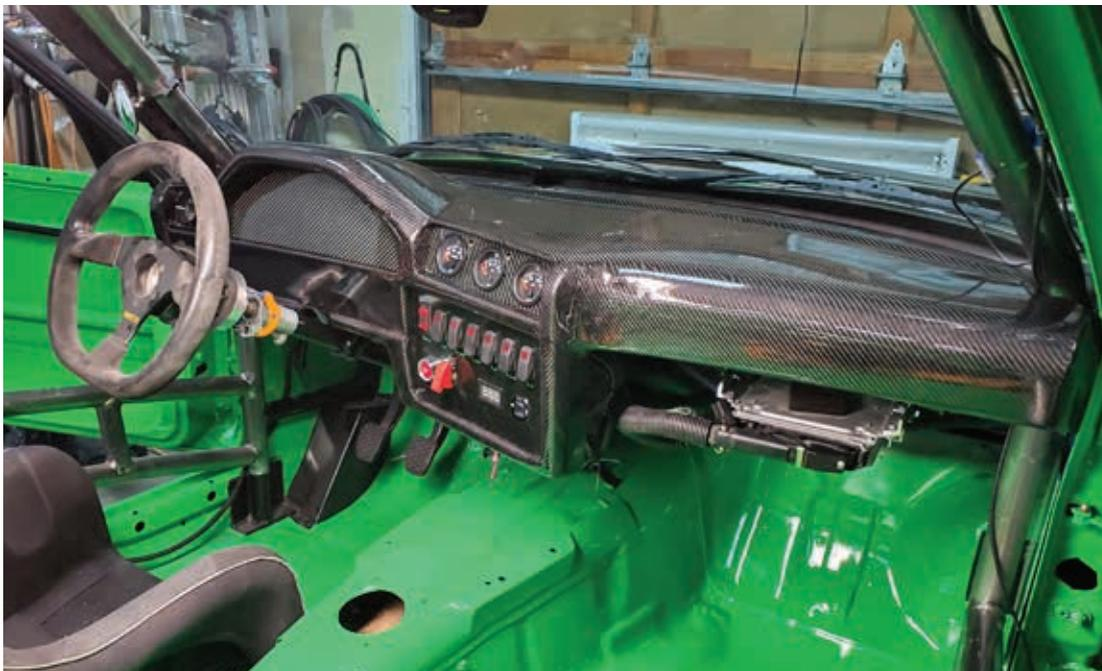
*The finished carbon skinned dash reinstalled.*
