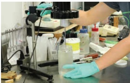
*The viscometer has a paddle which measures a sample's resistance to flow (viscosity). Each sample is tested for three minutes to ensure an accurate reading.*
