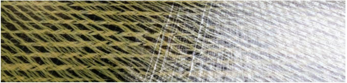
impact and abrasion resistance. Because of their high strength, they're frequently used in sailboat rigging. Honeywell Spectra fabrics tend to be more expensive, so might not be as readily available as other reinforcement fabrics in retail settings.
