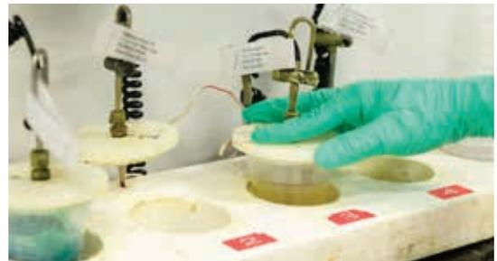
*The peak exothermic temperature is measured using 100 cc of epoxy in a standardized 120 cc beaker. A thermocouple connected to a computer analyzes the results.*
