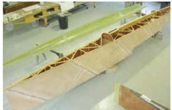
*The hull bottom and the trussing for the ama ready to be assembled. Shown above is the semicircular, fiberglass hull bottom which will be flipped over and epoxied to the plywood trussing section of the ama.*
