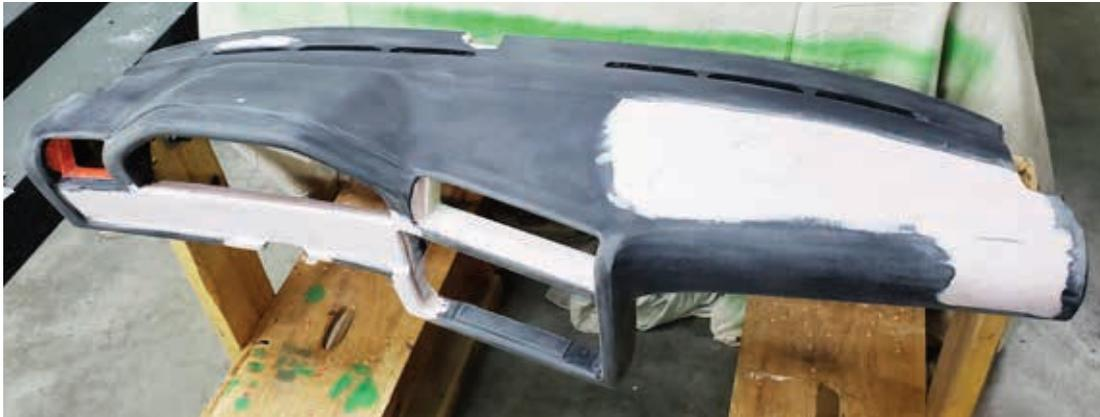
*The insulation was faired in with 105/207 thickened with 410 Microlight Filler.*
