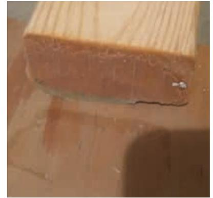
*This timber bonded unsuccessfully. You can see the shine of the epoxy on the bottom of the 2x4. Note that there are no wood fibers missing from the plywood panel in the top image or attached to the end grain in the bottom image.*
