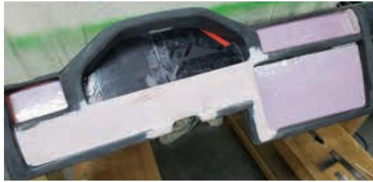
*Foam or cardboard backing blocks were inserted into each opening to mold a flange for remounting hardware.*
