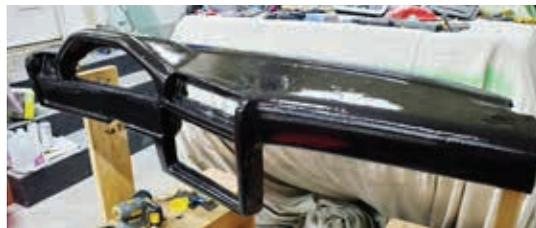
*A black pigmented coat of G/flex was applied to the dash before applying the carbon fiber fabric.*
