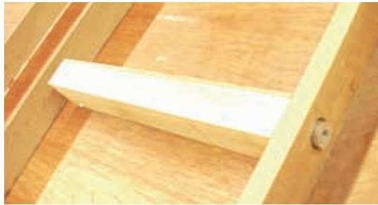
*The aluminum/wood assembly epoxied into the desired location in the hull.*
