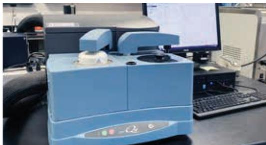
*The DSC is a very controlled environment for testing the exotherm of samples with intense sensitivity.*
