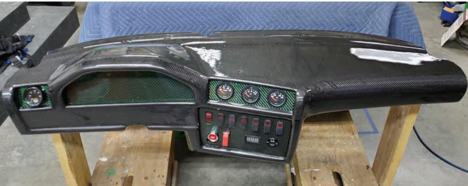
*The completed carbon skinned dash reassembled and ready for installation.*
