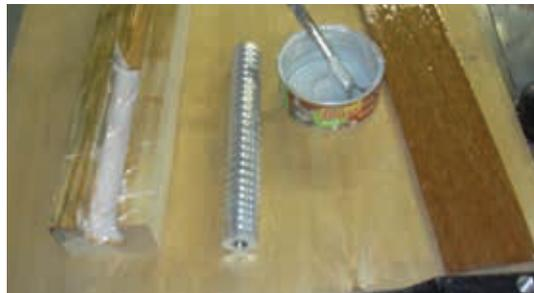
*The notched aluminum rod being bedded in its wood housing.*
