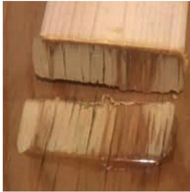
*An example of a successful bond. The bonding of the epoxy to the plywood was stronger than the bond of the wood fibers to one another. You can see the wood fibers still attached to the end of the 2x4.*
