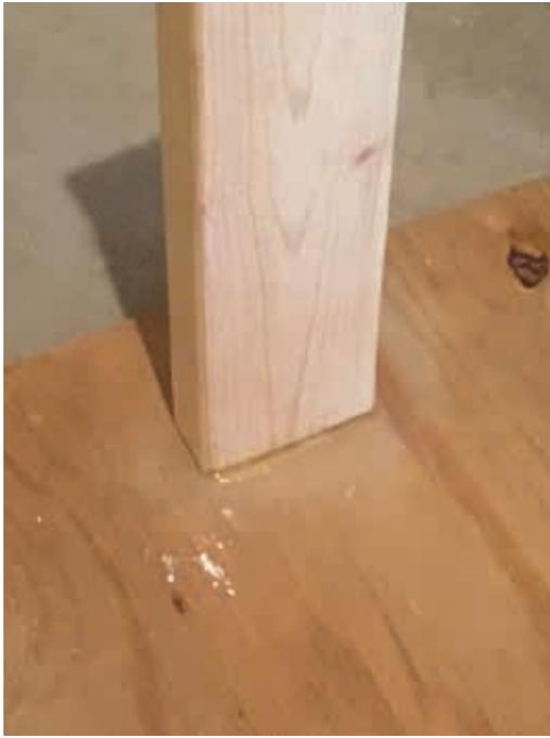
*An example of a home adhesion testing setup. The end of a 2x4 was epoxied onto the surface of a plywood panel and allowed to fully cure.*
