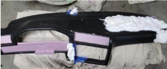
*Pink foam insulation board was used to fill in large flat areas. Expanding spray foam was used to fill in the shallower or more contoured areas.*
