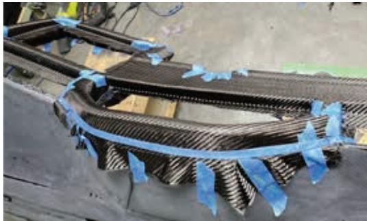
*With a coat of 105/207 applied, the front of the dash was covered with carbon fiber. Butt joints were created at the corners or seams to make them less visible transitioning onto the other surfaces of the dash.*
