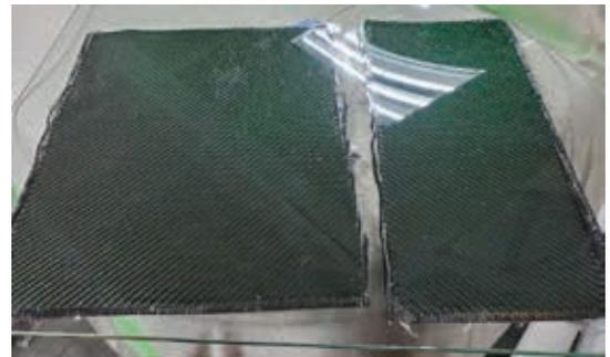
*Two of the panels for the switches and gauges. The finished surface was carbon with green metallic accents woven through the fabric.*
