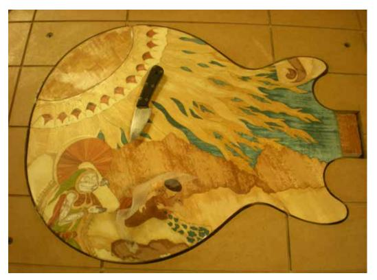
With the epoxy cured, the vacuum film was removed and the piece is now ready for sanding and detailing with a knife-tipped woodburning pen.
