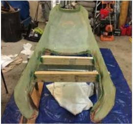
Because the loaned car body could not be altered, this female mold was created to build a second body that could be altered.
