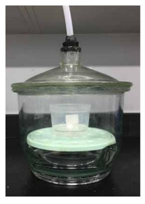
The second method is to put the epoxy in a vacuum chamber, which will quickly evacuate the air bubbles. Be sure not to pull so much vacuum that the epoxy starts lifting, which will look like it's boiling. Once you turn off the vacuum, slowly let the air back into the chamber. Opening the chamber valve completely at once can create a rush of air into the chamber, inducing air back into the epoxy.
