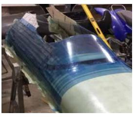
Using an old windshield and flash tape attached to the car body, the new cockpit shape begins to form.
