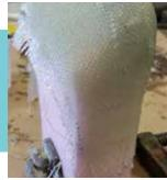
Fiberglass applied to the mold. Small pieces were overlapped to follow the contours of the part.
