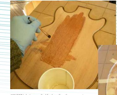
105/207 is being applied for bonding the marquetry work. Using 105/207 to adhere the marquetry and as the seal coat, gives the finished product a unified appearance.
