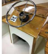
The wheel installed. The helm station is built of okoume ply with a black locust corner post and Cypress dash and shelf. The seats are cedar.
