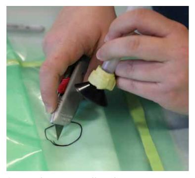
Connecting the vacuum port and line to the bagged laminate
