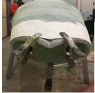
A scrap of curved fiberglass panel was the perfect piece to extend the nose of the car body to match the new profile.
