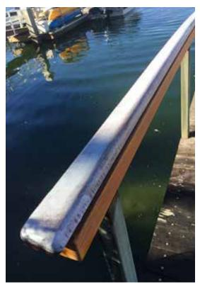
105/207 put on late in the day in cool weather. Temps down into the 50s with a heavy dew turned the epoxy milky. This was an extreme case of moisture exposure before being fully cured.
