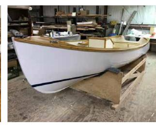
What a sweet sheer! The waterline was applied from plans. Often builders float the completed boat and mark the waterline location to paint later.
