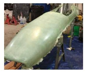
An exact copy of the borrowed car body was created from the female mold.
