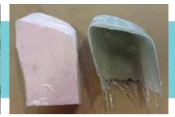
Mold removed from the cured epoxy/fiberglass part
