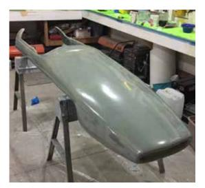
An old car body was loaned to be used as a plug to create a female mold.
