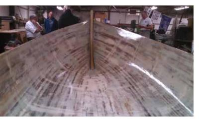
The hull off the mold and covered with fiberglass. The interior was faired before the fiberglass was applied.
