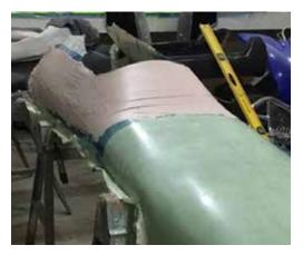
A fairing compound was applied over the flash tape to smooth the surface and stiffen the area. This will be sanded fair and sealed with epoxy.
