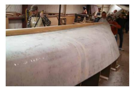
On the molds with the keelson added. Time spent fairing mold frames is time and materials saved in the fairing process. 410 Microlight filler added to WEST SYSTEM made for a nice fairing compound.
