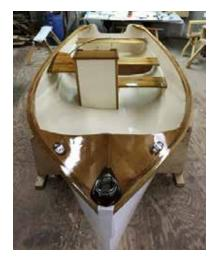
With the interior painted, the hardware was installed. It's important to seal all holes with epoxy after they are drilled.
