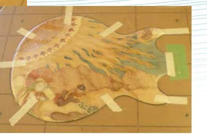
A vacuum press clamps the marquetry onto the guitar body with even pressure across the whole surface.
