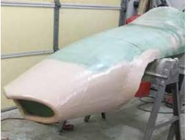
coat of epoxy, then applying a release agent to the epoxy, prevents this from happening.
