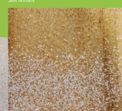
Texture built with a roller cover for aggressive nonskid.
