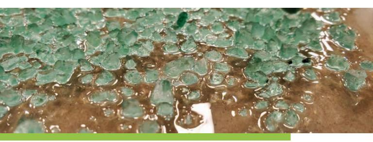
Rock salt used for the lost method of creating nonskid.
