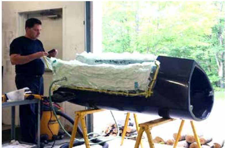
Vacuum bagging repairs on a bobsled.
