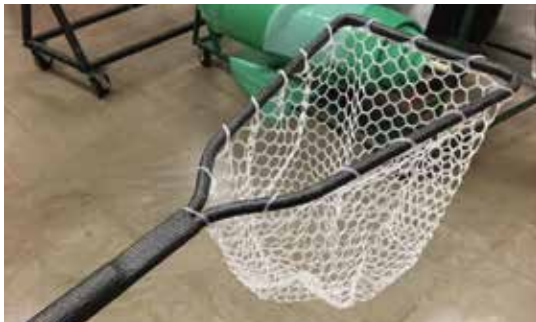
Carbon fiber landing net that was done as a senior design project
