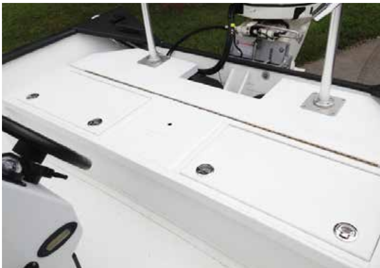
Finished rear deck hinge
