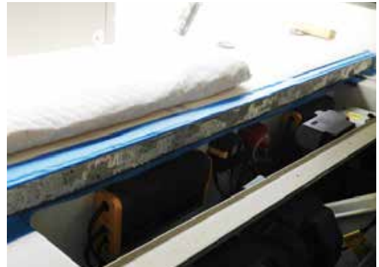
Prepped surface area on the boat side of the hinge
