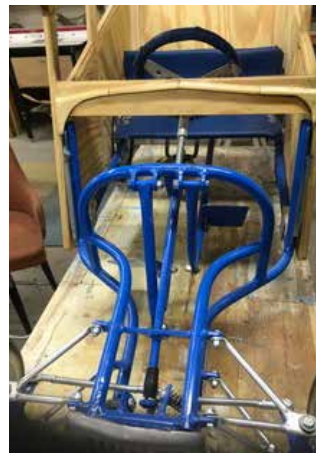
Right: The street rod pedal car was built from 3/4" steel tubing.
