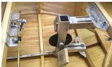
Above left: The steering wheel and pedal assembly
