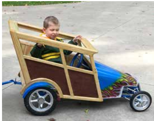
Car body is made with pine and mahogany veneer. The hood and fenders are painted sheet metal.
