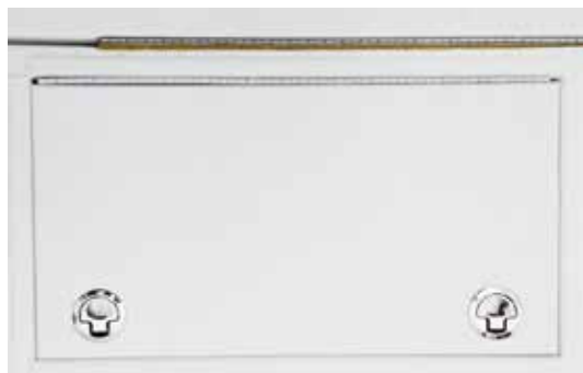
The reinstalled hatch ready for painting.
