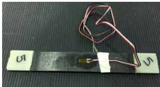
A unidirectional carbon tensile test specimen
