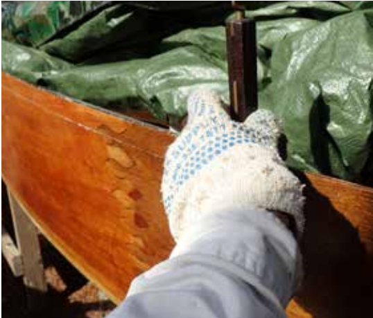
Marking the bottom edge of the gunwales with a scribe
