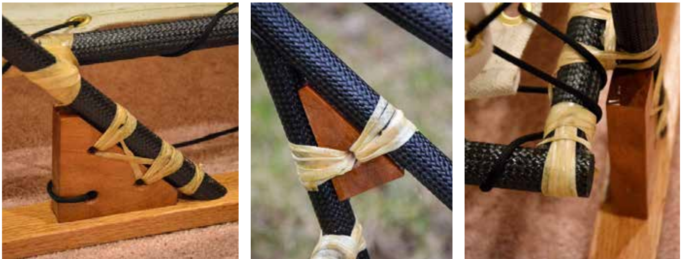
Composite rails and stanchions were lashed together with wet rawhide, which, when dry, results in tight but flexible joints. The hardwood blocks help provide support for the rawhide lashings.
