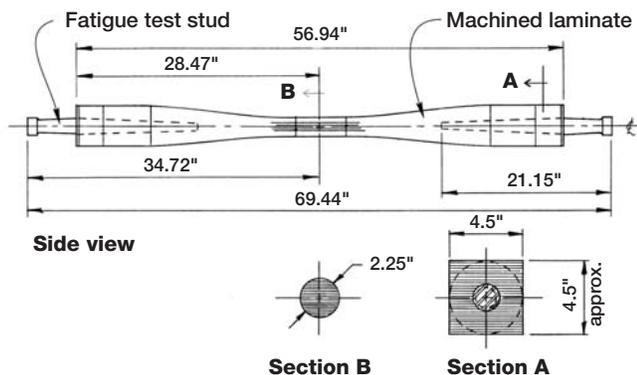
**Figure C-7** Detail of "dogbone" type fatigue test specimen.
