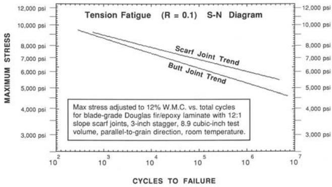
Figure C-9 Scarf joint and butt joint trend lines.
