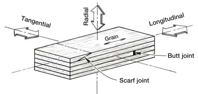
**Figure C-8** Reference Axes for Laminate Strength Measurements.
