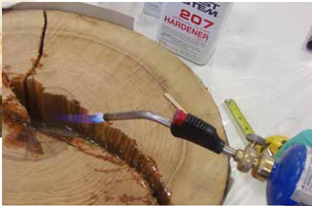
Bubbles rise to the surface of epoxy following a pour. Using a propane torch you can break the epoxy's surface tension, removing air bubbles. Using the multiple pour technique, the result is a 3½" deep casting of 105/207, free of bubbles.
