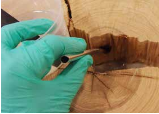
Brush one or two thin coats of epoxy onto the wood's surfaces and allow it to cure about 6 hours. To avoid sanding, don't coat higher than you plan to pour over the next 18 hours.
