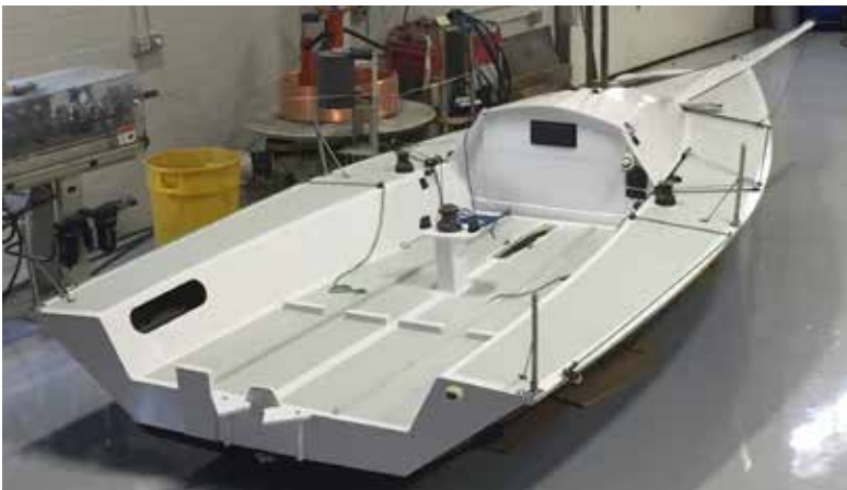
Non-skid painted and deck hardware reinstalled.
