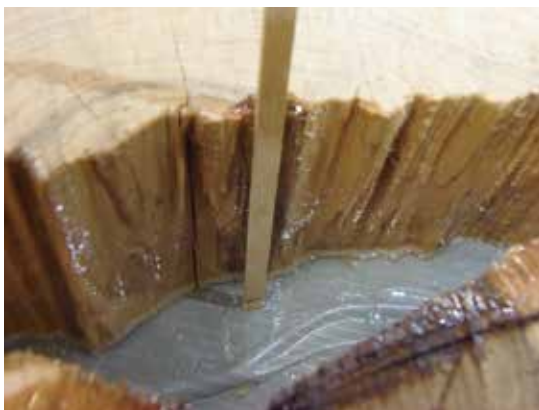
A stir stick marked at 1/4" will make it easier to measure the depth of your pour.
