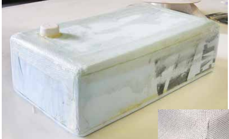
The edges of the foam box rounded over then reinforced with 731 glass tape.
