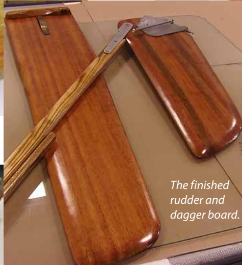
After three coats of epoxy were applied.
