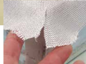
It's important to cut a pleat into the corner so the glass will lay flat.
