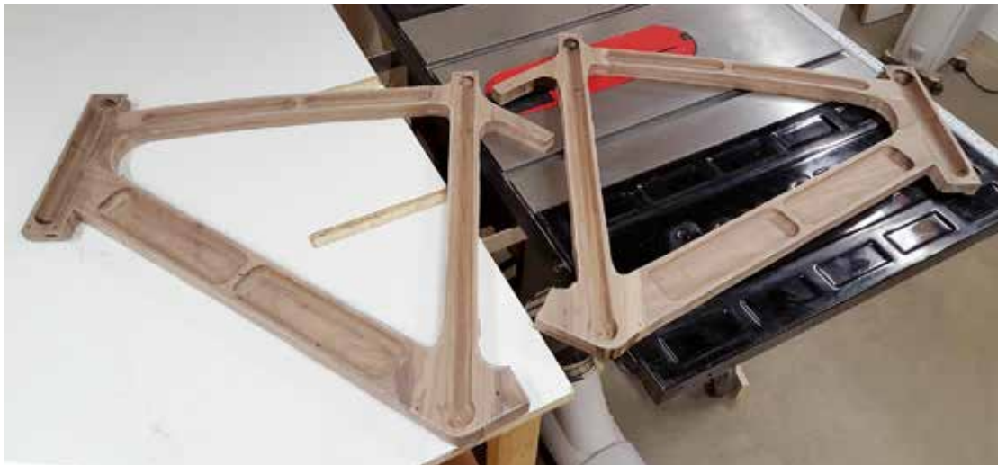
Excess wood trimmed away. Pockets routed for the steel inserts.
