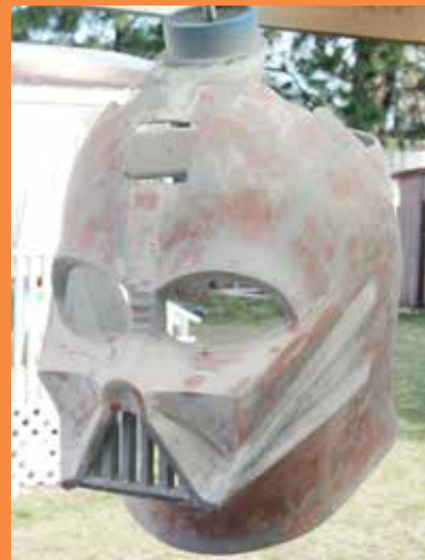
Bottom Right: The fiberglass shell after 105/206 and 407 filler has been applied and faired.
