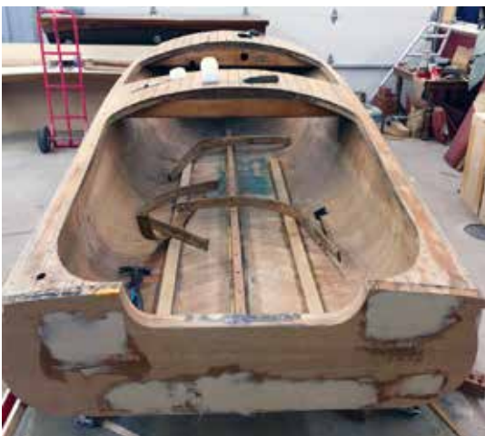
Transom faired before another layer of veneer is applied.
