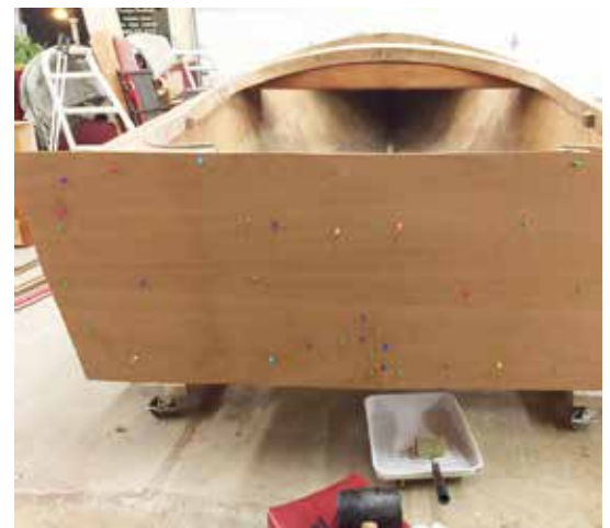
Transom veneer temporarily held in place using push pins
