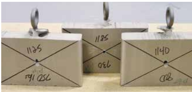
Hardware bedded in Azek boards and pulled until failure.
