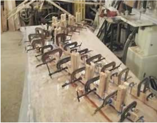
The laminates clamped onto the brackets while curing.
