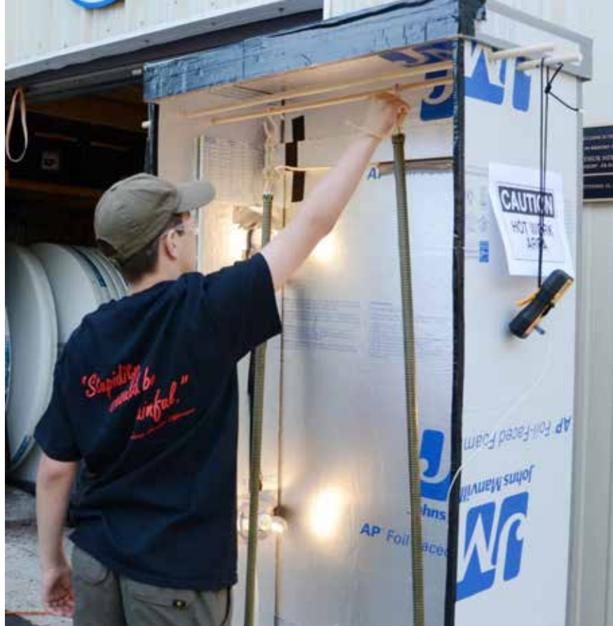
The cure reaction was accelerated by heating in an oven (home-built using insulation board and halogen lights) to allow the scouts to apply three coats of epoxy within the 8 hour day.
