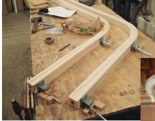
The laminates for the legs trimmed and sanded.
