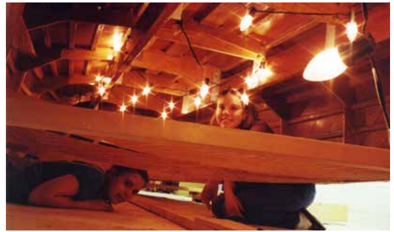
Mark's kids show off the incandescent Christmas lights they strung inside the hull to help make it easier to see the epoxy squeeze out.
