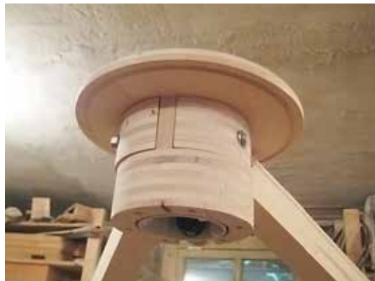
The fan hub assembled with the rooflet ready for epoxy coating and painting.
