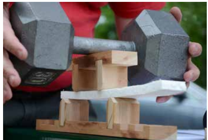
The composite panel supported over 30 pounds.
