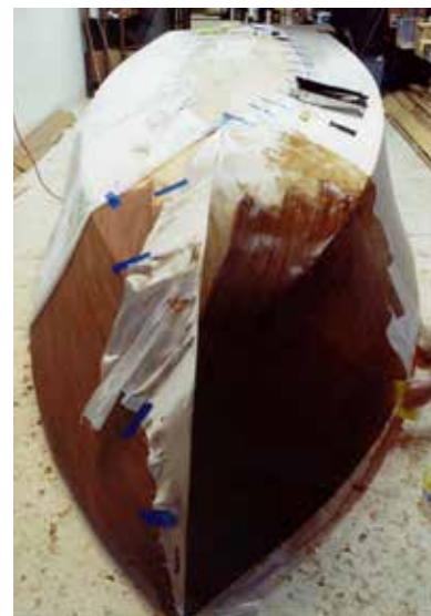
6 oz. fiberglass applied to the hull using the dry method
