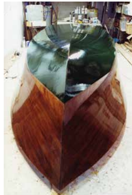
The hull finished, waxed and ready to be flipped and moved to the trailer for the rest of the build.
