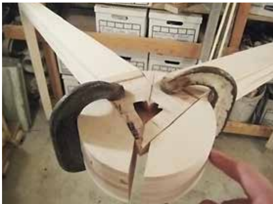
The fan hub clamped to the legs.
