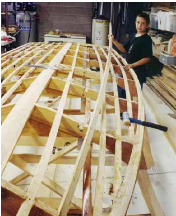
Mark's kids show off the incandescent Christmas lights they strung inside the hull to help make it easier to see the epoxy squeeze out.
