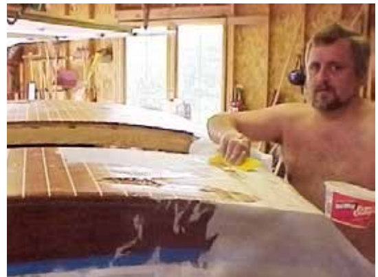
Mark applying fiberglass to the deck. It was 90°F when this picture was taken, but when using epoxy, gloves and a T-shirt are still strongly recommended.
