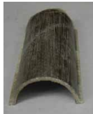
Cardboard tube fiberglassed and ready to be installed as a limber hole.
