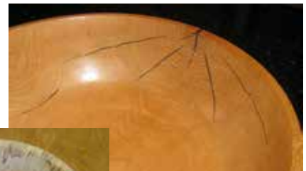
Turned pieces that had cracks filled with graphite powder creating the same effect as using 502 pigmented epoxy
