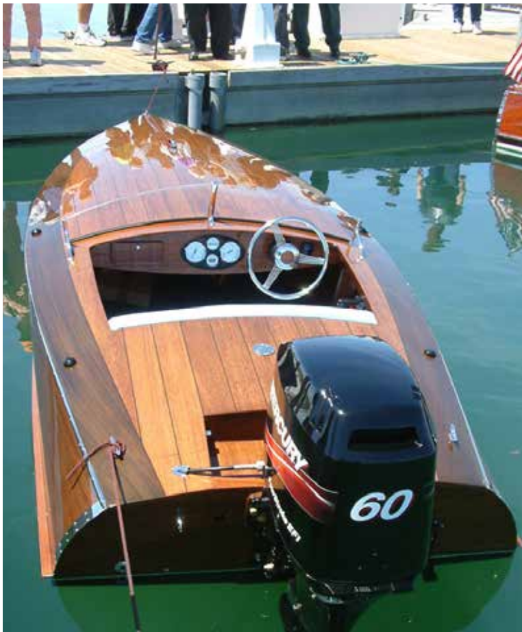
Even on wooden boats, proper fairing and finishing is important. Note the mirror like finish on RASCAL, a 14'10" runabout built by Steven Gembrowski. His build was featured in Epoxyworks 24.
