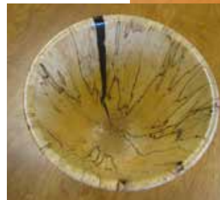
Turned pieces that had cracks filled with graphite powder creating the same effect as using 502 pigmented epoxy
