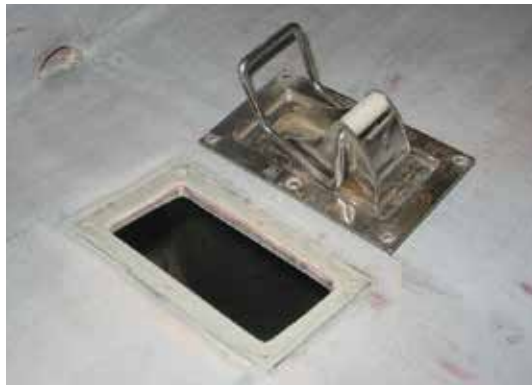
Andersen bailer ready for installation. In the top right corner is the limber through a watertight compartment
