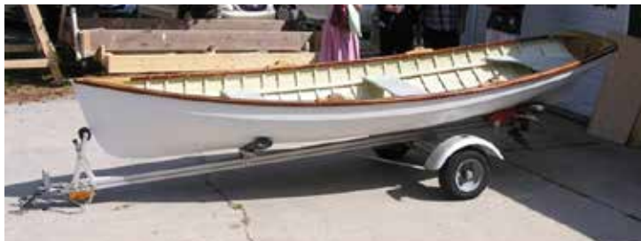
Students lofted, pulled scantlings and then built this replica of the 100-year-old Petoskey Boat Co. rowing dingy.
