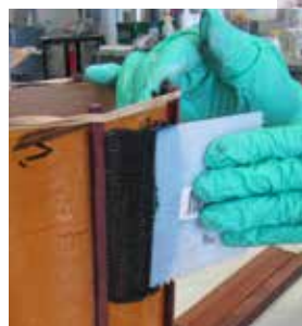
Black pigmented seams from "Drumming in Circles" in Epoxyworks 39
