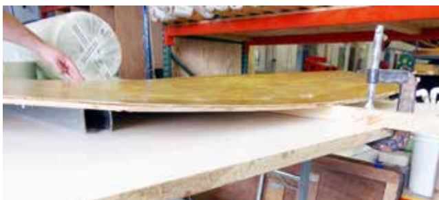
Applying a 1" rocker to the mold surface
