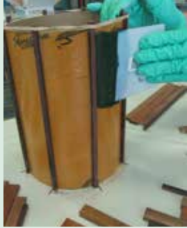
Using a notched spreader, apply thickened epoxy
