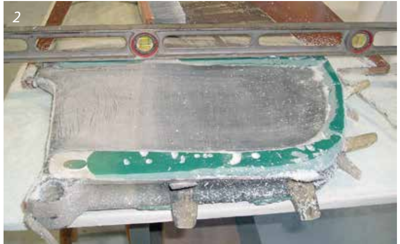
Leveling the top edge of the board
