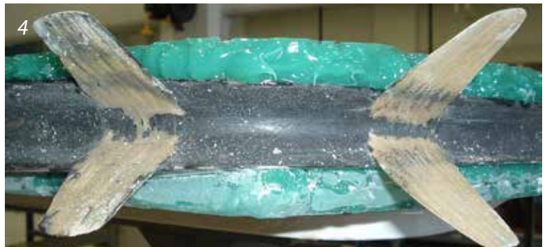
The trailing edge of the centerboard now complete.
