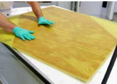
Mold surface: \frac{1}{4} " plywood with a sheet of \frac{1}{16} " thick G-10 glued on it
