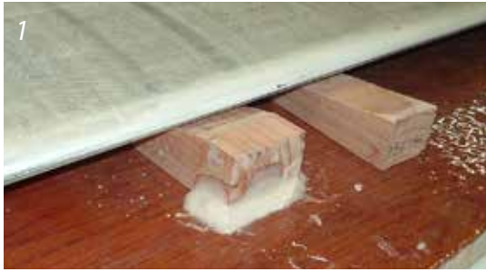
Wedges were used to level the centerboard and were held in place with G/5 Five-Minute Adhesive.
