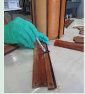
Dry fit then coat the strips and tube with unthickened epoxy
