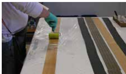
Top: Plywood jig to bend the brackets around Bottom: Wetting out the wood veneer
