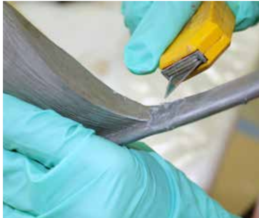
Left: Repair area wrapped in packing tape to form the shape of the stem.
