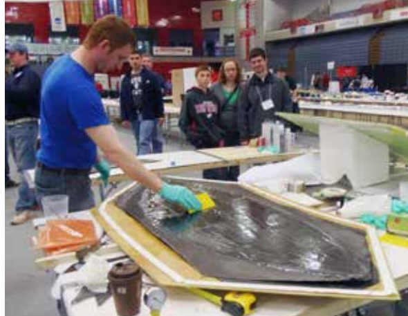
Vacuum bagging demonstration at MITES.
