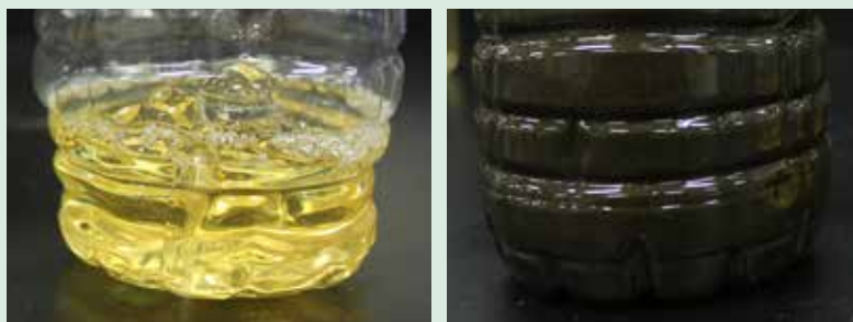
Left: A 1 inch deep pour (70 grams) of 105/206 in an 18 oz. bottle reached 410°F, cracked and deformed the bottle.
