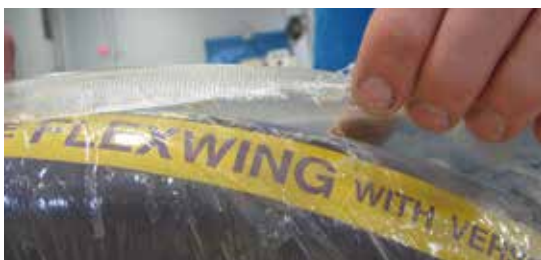
The cured fiberglass and epoxy easily pulls away from the mold surface.
