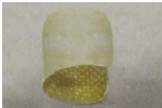
The Kevlar sleeve trimmed and sanded.
