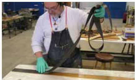
Top: Wetting out the carbon fiber reinforcing Bottom: Layering the carbon fiber on the wood veneer
