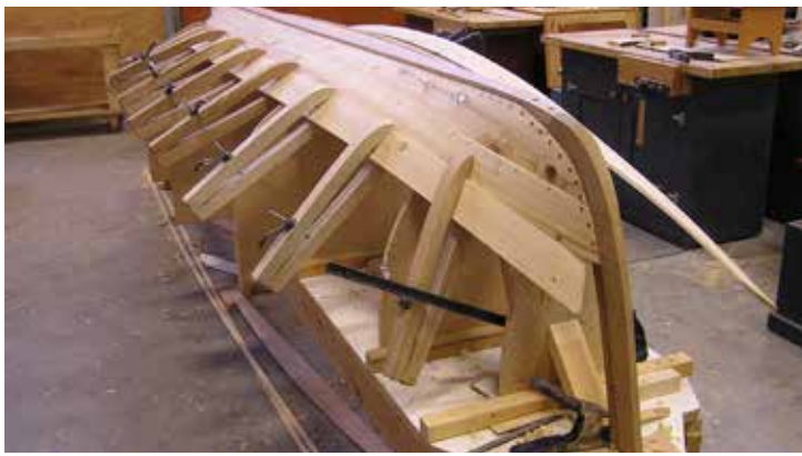
Left: This boat was found somewhere in Michigan and given to the school. The students had to work to get the boat back on its lines so they could take scantling measurements and loft the boat to make the replica.
