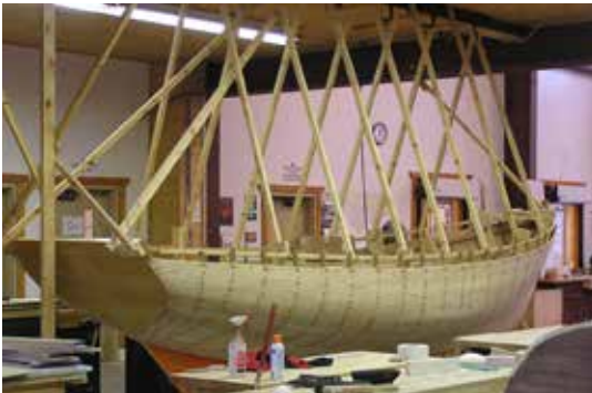
Top Left: The cedar getting sanded fair before getting coated with epoxy and glassed by second year students: (l-r) Troy Huesdash, Matt Edmondson, Kris Kindt and Del Jacobs. The Roberts Runabout is mahogany veneer over plywood. Bottom Left: The upright build is a Harry Bryan design named Katie. All first year students begin by learning to build using a "right-side up" technique.
