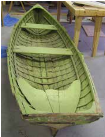
Left: This boat was found somewhere in Michigan and given to the school. The students had to work to get the boat back on its lines so they could take scantling measurements and loft the boat to make the replica.
