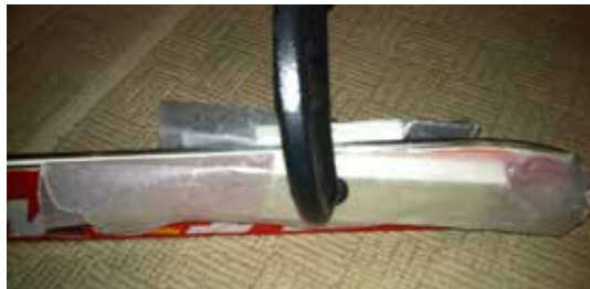
Clamped and curing at 68°F
