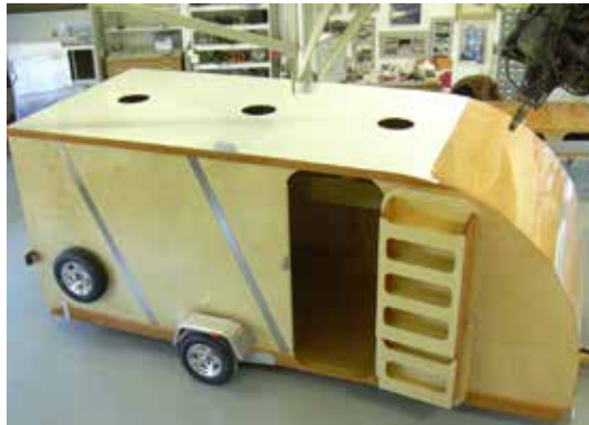
Storage compartments were built into the door for tools needed at the race track.
