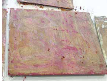
After the paint stripper was applied and lifted paint was removed, the surface was sanded with 60-grit.
