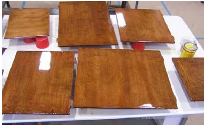
Finished door with 1/8" thick coating of 105/207
