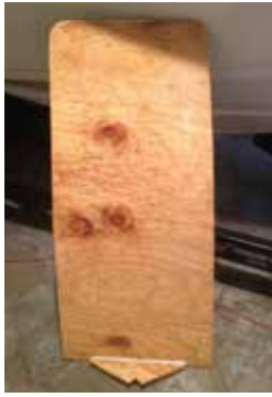
Left—New cabin sole with aft support frame Right—New cabin sole set in place
