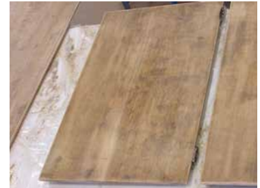
After the paint stripper was applied and lifted paint was removed, the surface was sanded with 60-grit.
