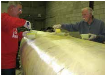
Painted with a birch bark pattern, the canoe receives another coat of epoxy.
