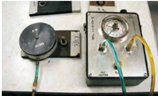
PATTI (Pneumatic Adhesion Tensile Test Instrument)
