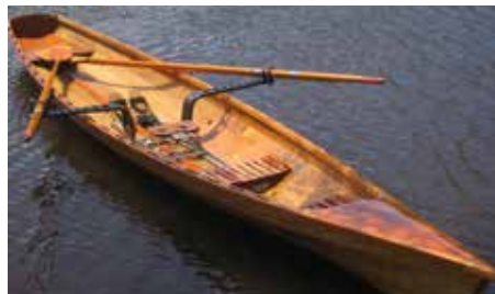
Rob Caveney built a 18' 9" Whitehall pulling boat named Indian using WEST SYSTEM Epoxy.
