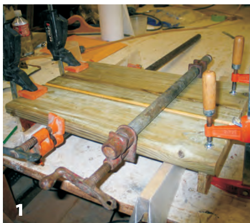
Figure 1—Alternating bar clamps and clamps at the end of the panel to keep it flat while the epoxy cures.
