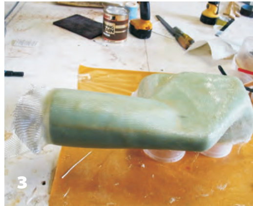
3—The fiberglass has cured over the Styrofoam mold before it is trimmed and sanded.
