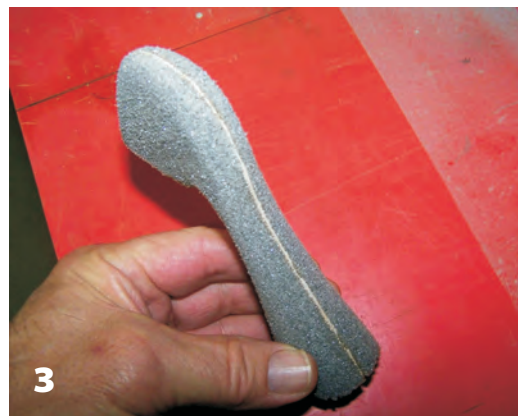
3—Then round over and smooth the corners with sandpaper.
