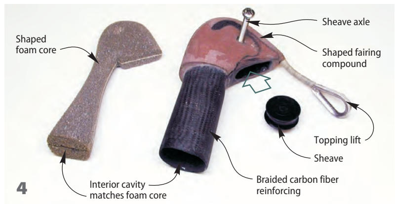
4—The nearly finished fitting with a duplicate of the foam mold. After the inside was cleaned out, additional fabric was applied to achieve the final exterior shape. The outside was faired and shaped before the topping lift and sheave were installed.
