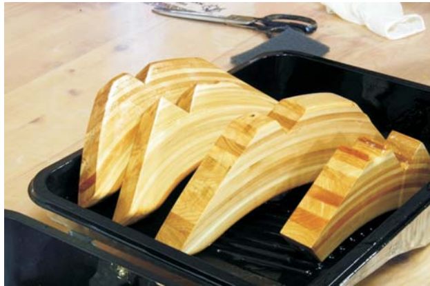
The laminated knees that support the deck on Sparks were sealed before installation. It would have been painful and hard to finish them in place. After dry fitting, the knees were dipped into thinned WEST SYSTEM 105 Resin/207 Special Clear Hardener and set to drain back into the paint tray. The excess was scraped off with a squeegee, rubbed in with a scuffing pad and wiped clean with a clean dry rag. The end grain was now sealed and ready for glue, and the surface was smooth and ready for the finish.
