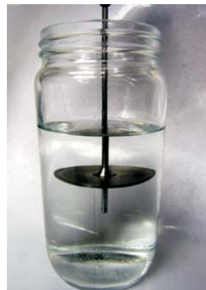
The rotational viscometer spindle suspended in a jar of resin.
