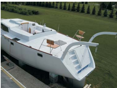
Earl Rentmeester of Green Bay, Wisconsin recently launched a 50' cold molded sailboat built from scratch using WEST SYSTEM Epoxy. He used 157 gallons of epoxy on this entire project, which took four years and ten months working full time to complete. Driftwood is a double headsail ketch with a pilothouse for inside and outside helms.
