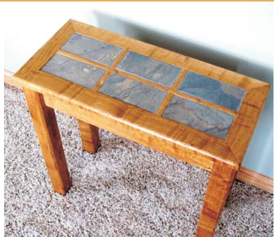
The finished table with three coats of varnish and the ceramic tile glued in place—with G/flex.
