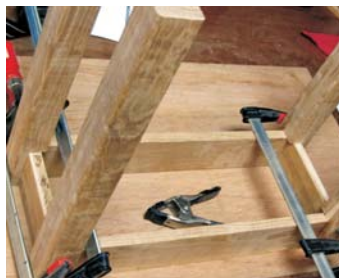
The legs, frame and top were assembled with G/flex 655 only.
