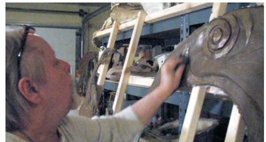
4. Buffing with steel wool exposed the bronze powder.
