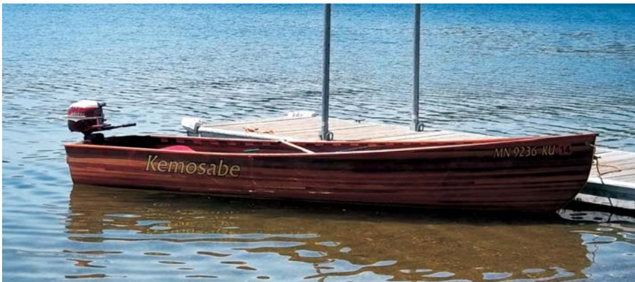
Jack Sommersness built this strip-skiff name Kemosabe . The hull is cedar, transom is mahogany, gunwales and seats are mahogany and black walnut. Sommersness is from Hutchinson, Minnesota.
