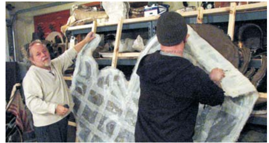
3. The silicone mold was peeled from the sculpture.
