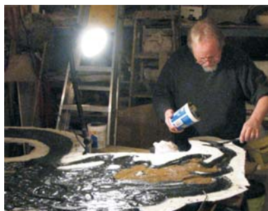
2. Epoxy/bronze mixture was buttered into the silicone/plaster mold.
