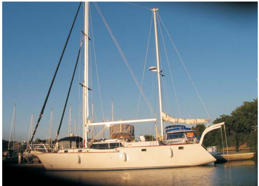
Earl Rentmeester of Green Bay, Wisconsin recently launched a 50' cold molded sailboat built from scratch using WEST SYSTEM Epoxy. He used 157 gallons of epoxy on this entire project, which took four years and ten months working full time to complete. Driftwood is a double headsail ketch with a pilothouse for inside and outside helms.
