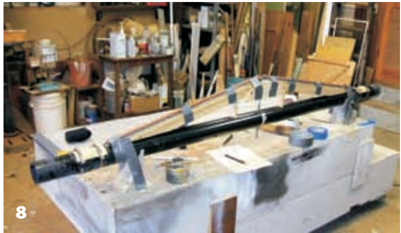
8—Carbon beams were purchased from Ben Hall and then a carbon dolphin striker was added to the front beam.
