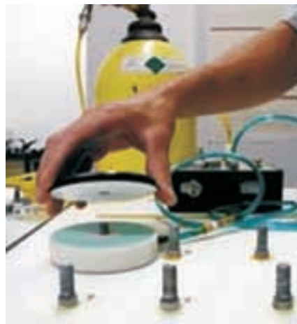
The Pneumatic Adhesive Tension Testing Instrument, or PATTI device, uses compressed air to inflate a bladder that lifts a metal stud glued to a substrate. A gauge measures the tensile force required to break the bond.
