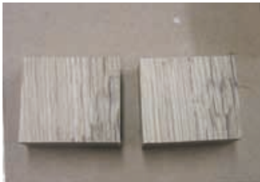
Here are two raw sample pieces showing the sawn surfaces before sanding to 80-grit.
