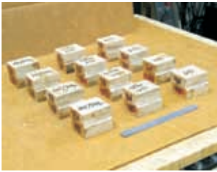
Above—White oak, single lap shear test specimens that have been prepared for the ASTM D905 short block shear test.
