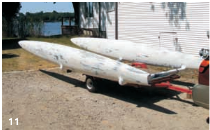
11—The faired catamaran upside-down on a trailer. Gluing the beams to the hulls rather than bolting them on resulted in a very stiff platform.
