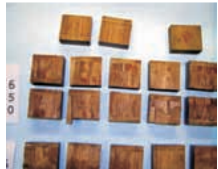
No surprises here-both the Six10 and G/flex 650 failed the wood extensively after six weeks of accelerated environmental cycling. These samples gained 16% moisture each time they sat in the hot humid environment and dried to a level 2.11% below the original moisture content coming out of the dry hut. The moisture content was 1.59% above the initial room temp/ambient humidity value at testing. The original control MC block which had been dried to -4.44% for testing sat out at room temperature in our shop here in mid-Michigan for the entire six weeks and gained back 0.77% moisture during that period.
