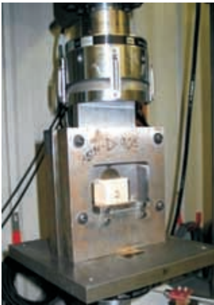
Below—The ASTM D905 test in progress. The test fixture is designed to minimize peel by presenting the shear force on the specimen parallel to the glue joint.
