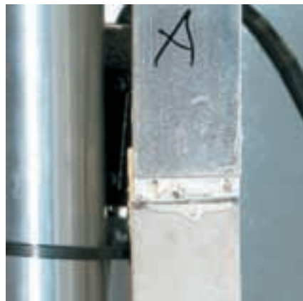
Below—The same sample after a shear failure of the adhesive.
