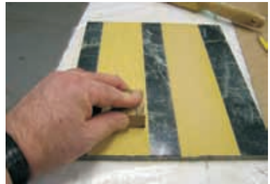
All the surfaces to be bonded were sanded with 60-grit then 80-grit on a marble tile to ensure flatness.
