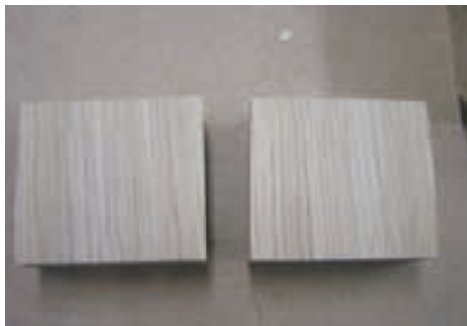
This is the finished sanded surface. Before glue was applied, each surface was also wiped with an isopropyl alcohol pad.
