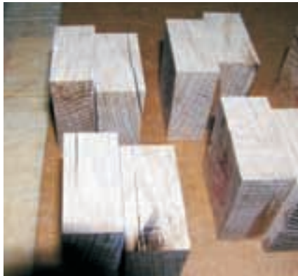
Here we see some of the damage to the oak blocks after the sixth week. We can also get an idea of the affect grain dive can have in these samples. Do not confuse the saw marks on the ends for the grain.
