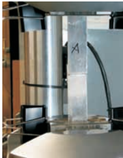
Above—Single lap shear sample in the test machine. The sample is two aluminum plates glued with a 1/2" overlap.
