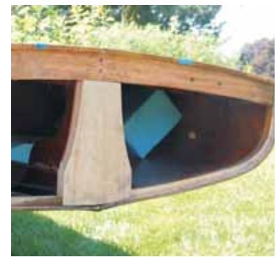
Left—The transom gusset clamped with a handy 4 x 4.
