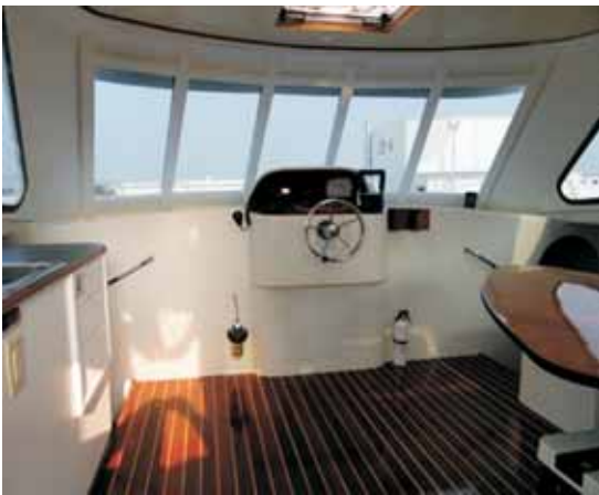
Ion's roomy main cabin. The instrument panel and hood and the table were built by Watson in Bay City and installed in the boat as construction progressed.
