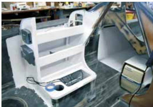
Interior galley area looking aft toward the two bunks under the cockpit. The interior was coated with white tinted epoxy before the deck was installed.
