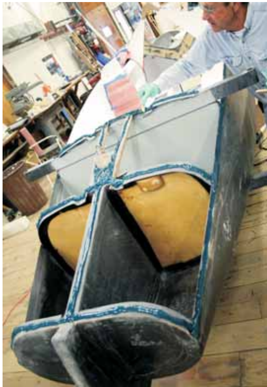
Interior galley area looking aft toward the two bunks under the cockpit. The interior was coated with white tinted epoxy before the deck was installed.
