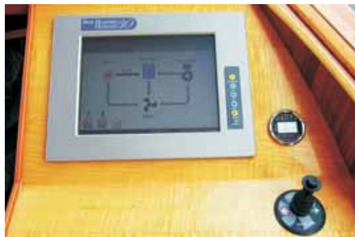
Next to a depth gauge, the computer's touch-screen interface displays all of the boat's systems. With the boat stopped, the display shows 200 kW directed to the batteries.
