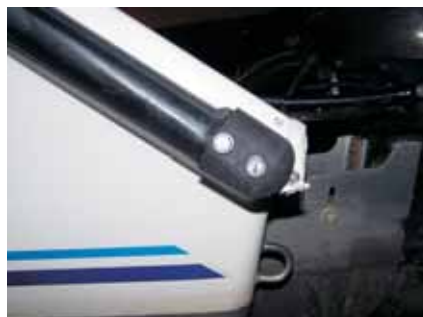
The finished rail cap installed.
