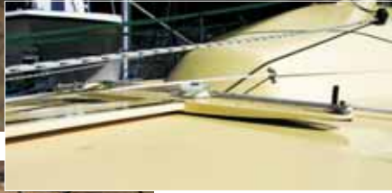
Left —The bowsprit is hinged at the bow and attached to a crossed line at the base of the cockpit (above) which will allow it to pivot 30°.
