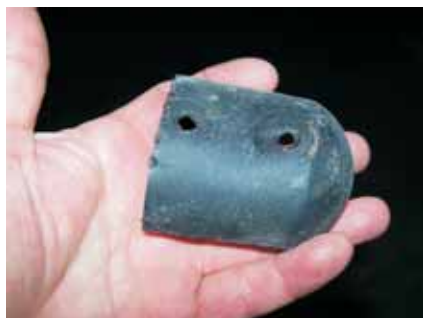
The finished rail cap.
