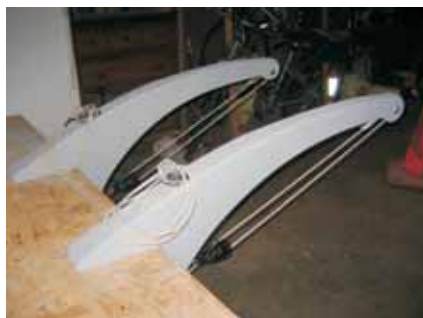
Nearly completed davits with primer applied. Note hoist line exit from top of the davit.
