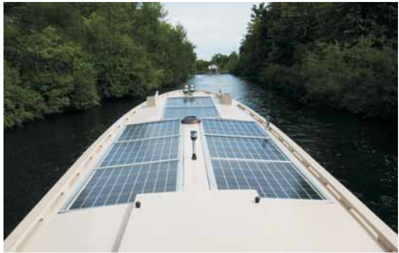
The eight Kyocera solar modules on the roof of Sparks , capable of producing 400 watts at 48 volts, are her primary source of power.
