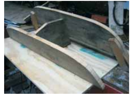
The foam with reinforcement on only one side was then placed over this male form and glass was added to the outside surface.
