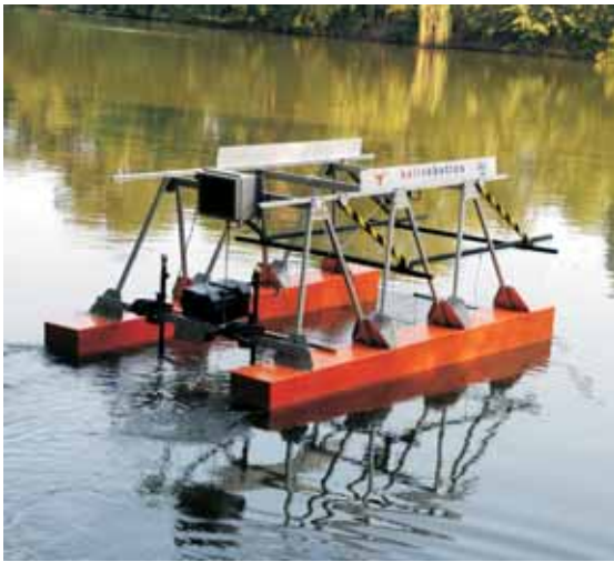
The remotely operated vehicle (ROV) scoops floating debris from the water's surface and collects it for removal.
