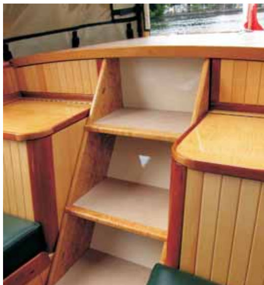
Left—The white cedar paneling on either side of the aft stairs is trimmed with cherry.
