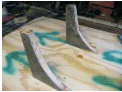
The gusset-like forms guided the tight radius. They're connected to my workbench which supports the flat section of the hood.
