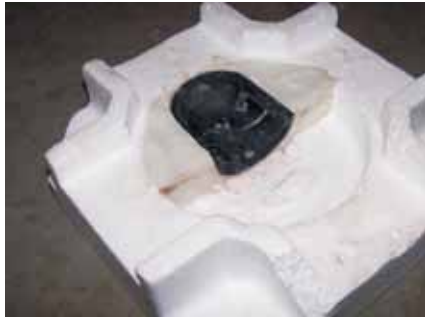
The existing cap was used to make a female mold in the thickened epoxy.
