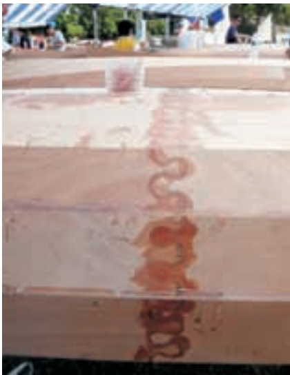
The very practical, puzzle joints make it easy to turn short planks into long planks.
