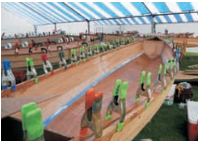
All of the inwales and outwales are glued, clamped and left to cure overnight. As the saying goes, "you can't have too many clamps."
