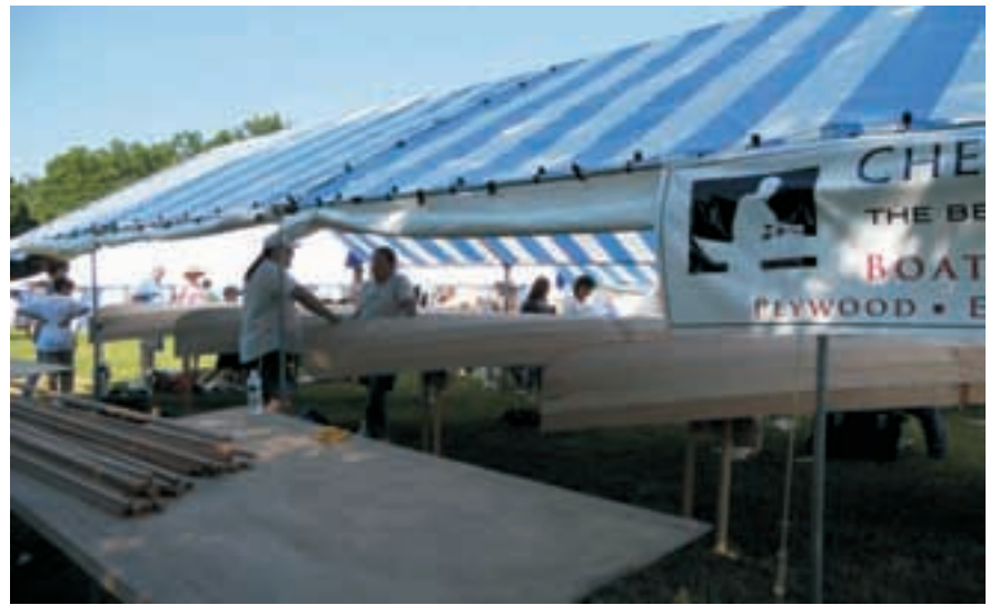
With the copper stitching removed and the outer lap joints filleted, the hulls are ready to be rolled upright again to install the inwales and outwales before the end of day two.
