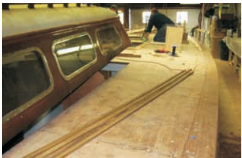
The deck house being fitted to the new deck.
