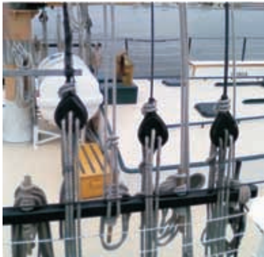
Figure 1—Traditional black locust deadeyes on the schooner Appledore IV . Deadeyes are used in pairs to tension the shrouds which hold up the mast.
