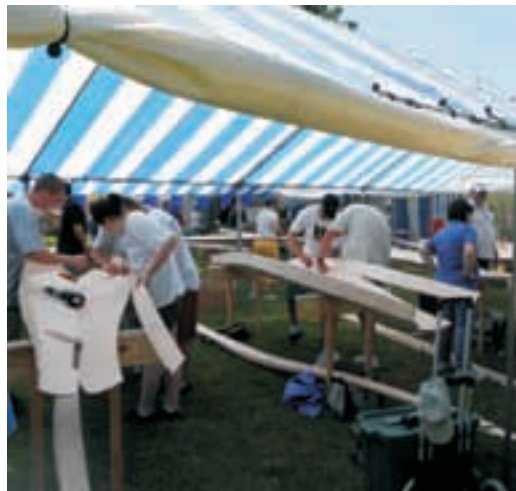
Nine families begin the building process by stitching the first strakes together with copper wire.
