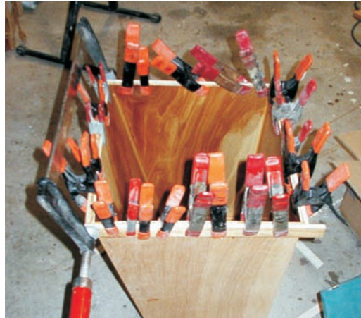
The wooden lip being attached to the basket (left) and a detail of the finished lip (above).
