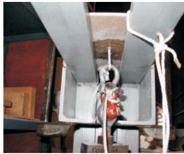
The extraction device with a digital load cell (left) that recorded the pull off strength of soft pad eyes glued to a fiberglass laminate (right).
