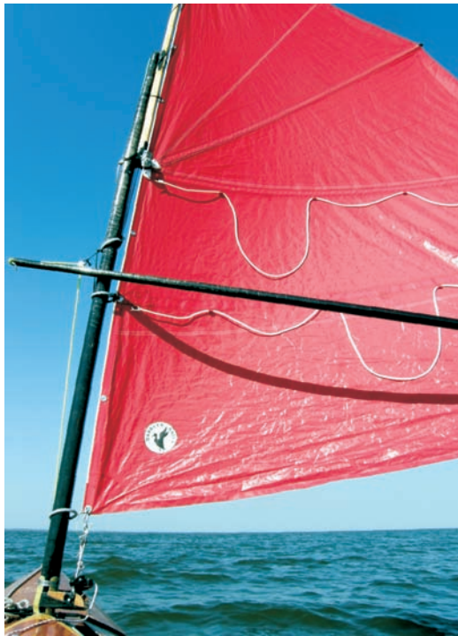
The unique “batwing” gunter rig on Hugh Hor- ton’s Bufflehead .
