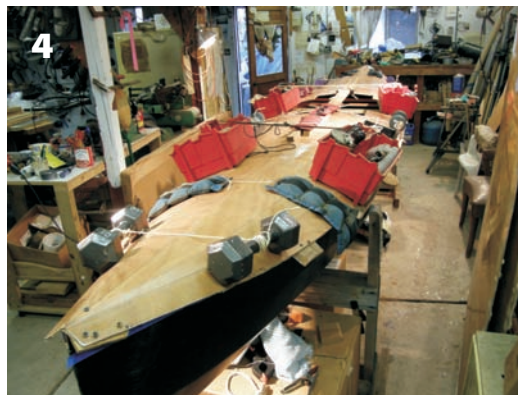
4—A deck being glued to a hull in Hugh Horton's shop. This bufflehead will be Jim Renouf's Eden.
