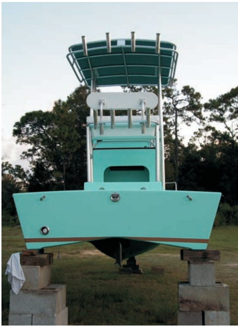
Joe Finn of Storm Port Boatworks, Homosassa, Florida, has launched the Oyster Cracker, a shallow draft, diesel powered flats boat. Joe says, "Lots of WEST SYSTEM® Epoxy went into this build. The rocks up here take their toll on props and boat bottoms." This design is based on W. Atkins Rescue Minor. She will run in 8" of water and gets 270 miles to a 9 gal tank of fuel. The boat was built right side up in a jig and is polished off with a yacht finish and mahogany trim. Storm Port Boatworks, 352-628-2983.
