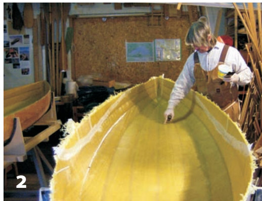
1,2,&3—Boat builder Skip Izon, of Grand Bend, Ontario, takes a Bufflehead hull from the cutout strakes and mold, to wetting out Kevlar on the interior of one Bufflehead and wetting out carbon fiber on the exterior of a second. This one will become Hugh's Bufflehead.
