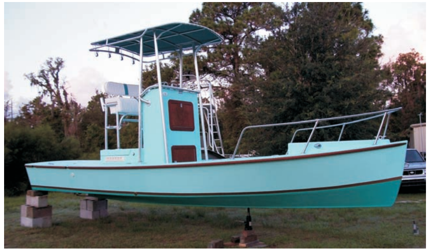
Joe Finn of Storm Port Boatworks, Homosassa, Florida, has launched the Oyster Cracker, a shallow draft, diesel powered flats boat. Joe says, "Lots of WEST SYSTEM® Epoxy went into this build. The rocks up here take their toll on props and boat bottoms." This design is based on W. Atkins Rescue Minor. She will run in 8" of water and gets 270 miles to a 9 gal tank of fuel. The boat was built right side up in a jig and is polished off with a yacht finish and mahogany trim. Storm Port Boatworks, 352-628-2983.
