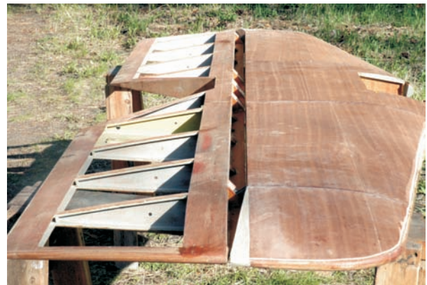
The newly covered stabilizer is temporarily attached to the elevator to check the fit of balsa blocks epoxied to the ends of the former. Both parts have been rebuilt using WEST SYSTEM Epoxy.
