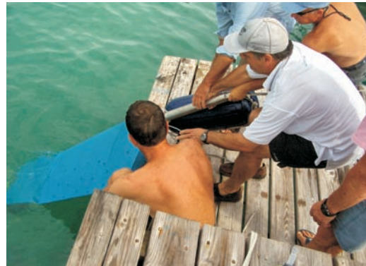
Pulling the 160 lb, 9'-long rudder onto the dock after it was removed from the boat while it was still in the water.
