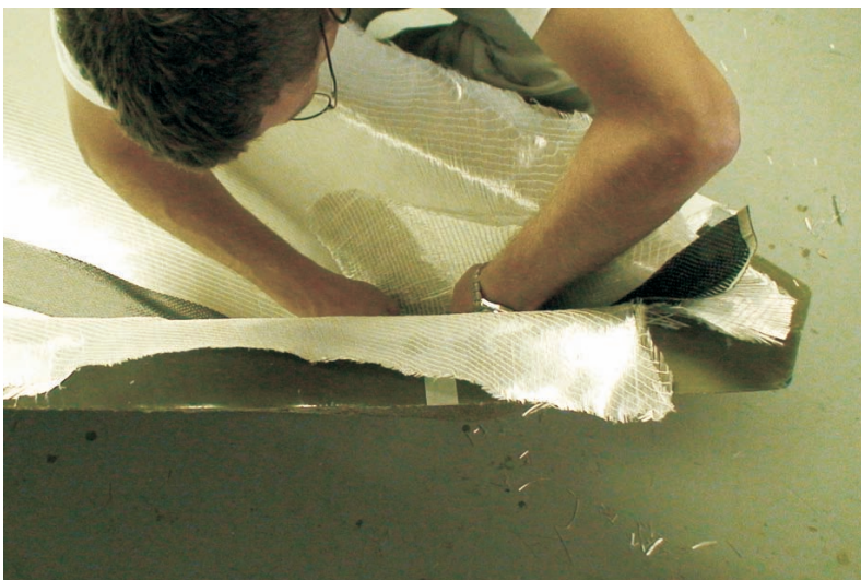
Alan Gurski installing layers of glass and carbon fiber tape into the mold for his resin infused version. He used two layers of 737 Biaxial Fabric, a thin foam core sandwiched between layers of 703 Unidirectional Carbon Tape followed by one more layer of 737.
