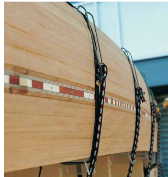
Below—Sections of clear polycarbonate tubing embedded in some accent strips available from Canadian Canoes glow as light shines through from the backside.
