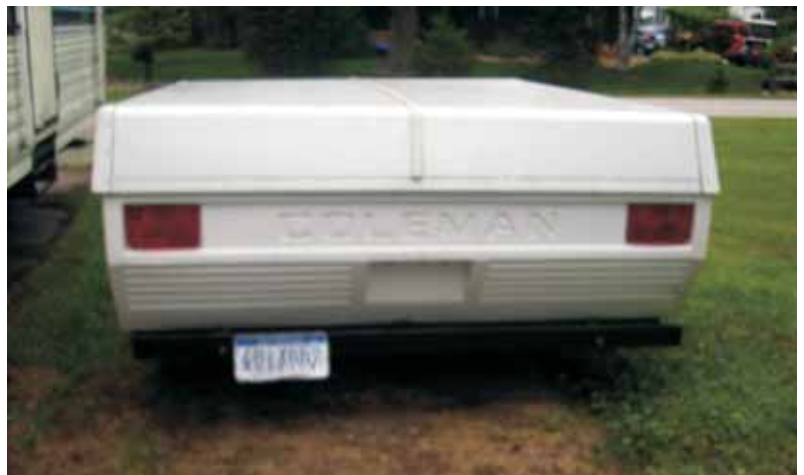
The repaired panel is back in place on the camper. A coat of Krylon Fusion™ textured, plastic-compatible paint completed the repair.
