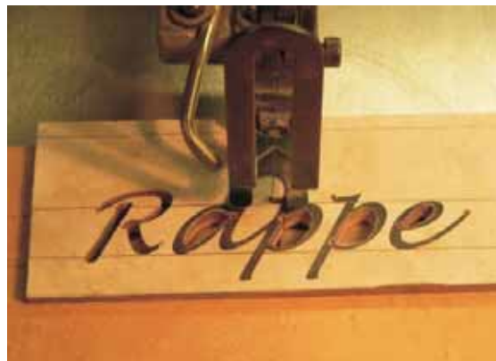
The scroll saw setup shows the enclosed portions of letters and the "R" have been cut out. The blade has been fed through \frac{1}{16} " hole ready to cut out the "ap."
