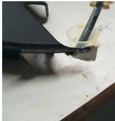
3—Fixing the broken tab with G/flex 655 and flame treating.
