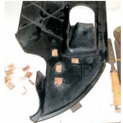
2—The test showed which combinations of glue and prep worked best.
