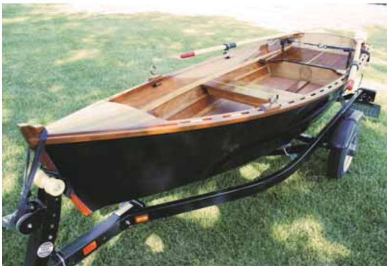
The interior was left natural wood—seats, bow deck and gunwales are mahogany with Sitka accents. The hull is painted with House of Color™ Midnight Blue Pearl.
