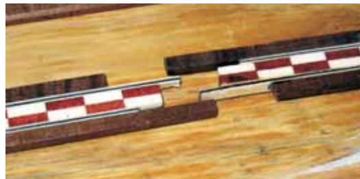
Below—Sections of clear polycarbonate tubing embedded in some accent strips available from Canadian Canoes glow as light shines through from the backside.
