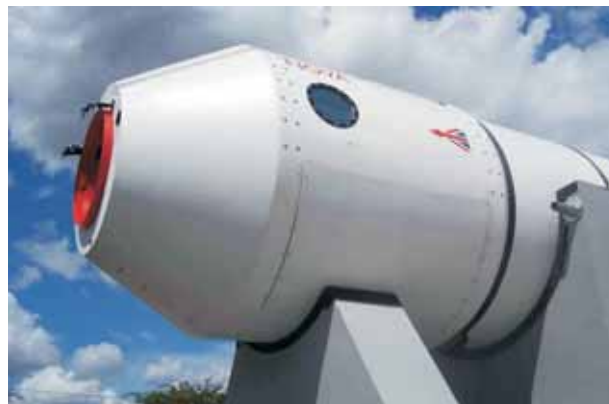
The unmanned capsule will be ejected mid-air and is designed to land safely by parachute.
