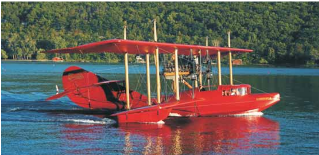
A 72' wingspan reproduction of the 1914 Curtiss flying boat America was completed by the museum's Restoration Shop crew in early September 2007.
