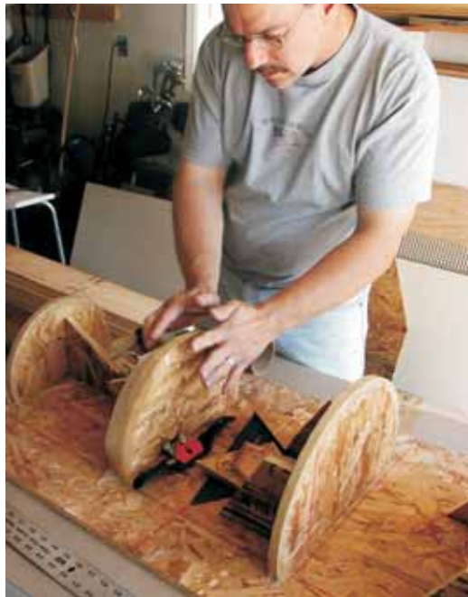
Bob covers the mold frames with tape so glue used to hold the wood strips together will release from the mold.
