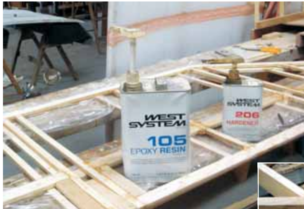
The 1910 Albany Flyer is the current construction project. Instead of the animal glues used in the original, this reproduction uses WEST SYSTEM Epoxy.
