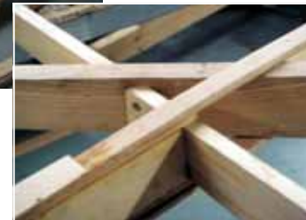
The 1910 Albany Flyer is the current construction project. Instead of the animal glues used in the original, this reproduction uses WEST SYSTEM Epoxy.
