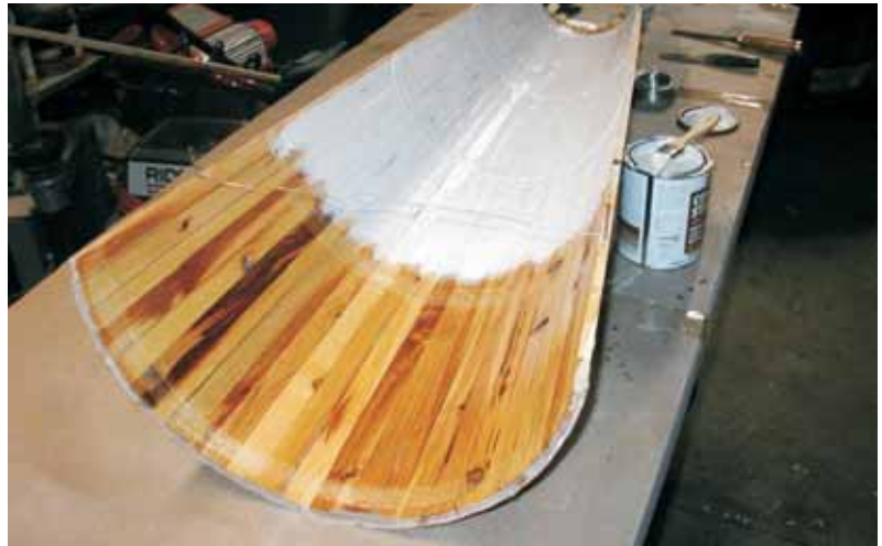
The insides of the completed tower halves were painted with a white latex primer so that a single low voltage light bulb would reflect inside the tower.
