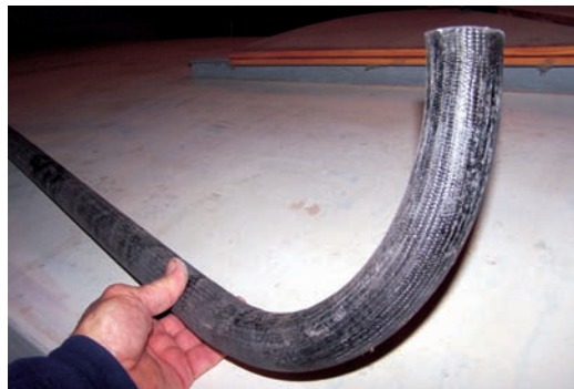
Figure 5 —A tapered tube section joined to a curved section.
