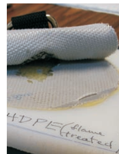
Figure 3—Another example of a pad failure in Phase II testing.
