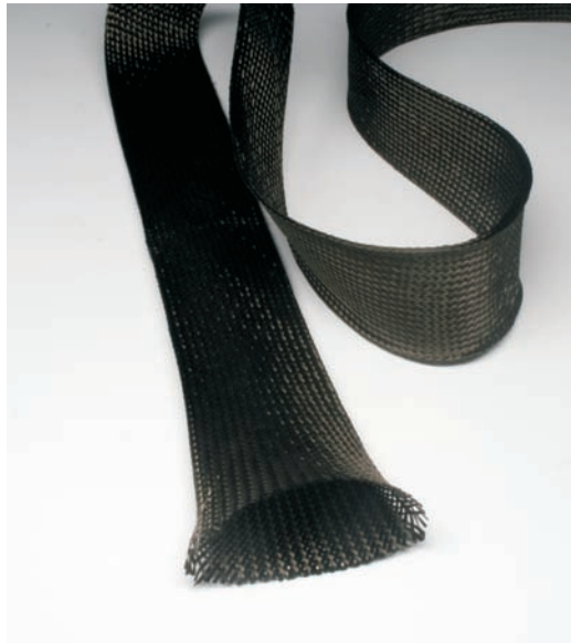
Figure 1 —Typical braided tube of carbon fiber. The length-to-diameter ratio can be altered like a Chinese finger trap.
