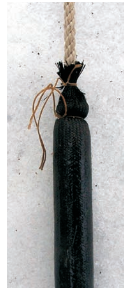
Figure 2—Making a composite tube using foam pipe insulation, rope, and monofilament fishing line.
