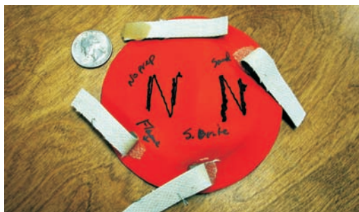
Figure 1—Phase I, gluing upholstery fabric to the D-ring pad to test G/flex adhesion.
