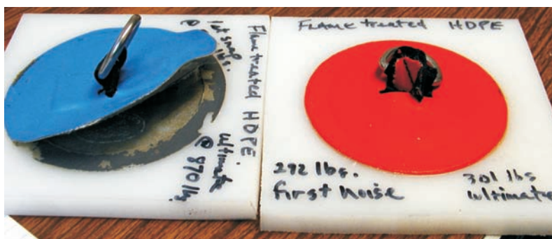
Figure 2—Results of Phase II tests. Failures occurred in the D-ring strap or in the pad itself.
