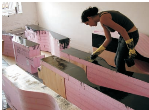
Figure 2 —Left, a worker coats one of the foam and wood laminated chaise lounges with epoxy tinted with graphite powder.
