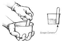
Figure 3 Stir resin and hardener together thoroughly—at least 1 minute, longer in cooler temperatures.
