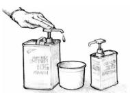
Figure 2 Dispense the proper proportions of resin and hardener.
