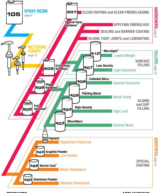
Start with 105 Epoxy Resin, the basic ingredient of all WEST SYSTEM Epoxy compounds. Use 300 Mini Pumps for convenient and accurate metering.
