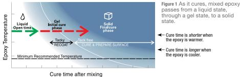
passes from a liquid state, through a gel state, to a solid
