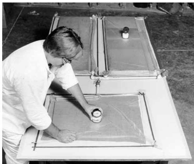
Figure 3-1 A flat, smooth surfaced table is a versatile mold for a wide variety of projects. Several lay-ups can be completed at the same time.
