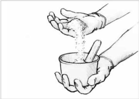
Figure 5-7 Blend in small handfuls or scoops of the appropriate filler until the desired consistency is reached.
