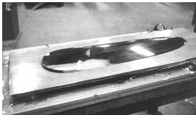
Figure 3-4 A plug for a rudder, with the shelf positioned at the rudder centerline, is waxed and ready for the application of the mold half.
