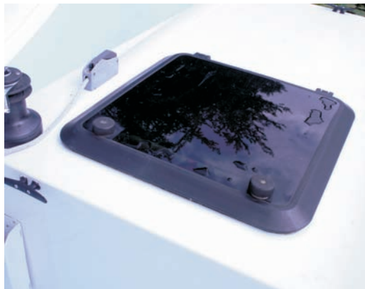
← Photo 7 —Clean off excess epoxy from the perimeter of the flange with the flat end of an 804 Reusable Mixing Stick.
