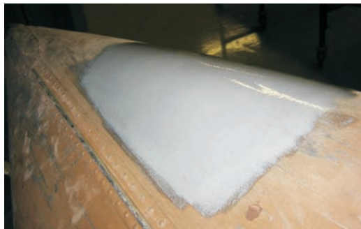
Photo 9 —A mix of G/flex 650 and 503 Gray Pigment was applied as a sealer/undercoating and a bit of camouflage.
