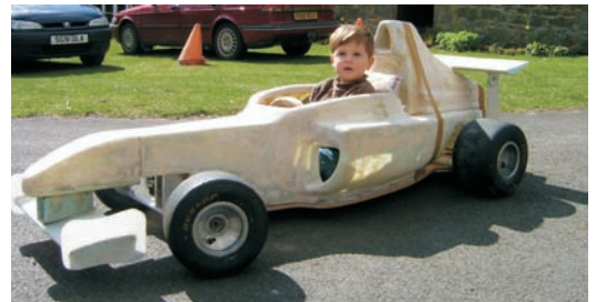
Bottom—The component body parts are assembled on the chassis. The Formula 1 is ready for a quick test drive before final finishing and a couple of coats of Ferrari red paint.
