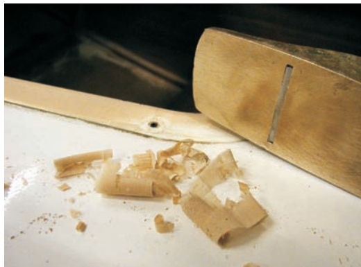
Photo 2 —One side of the new larger hatch was in the same location as a side of the old hatch. The low-density epoxy/410 Microlight mixture along that edge was easily removed with a low-angle block plane.
