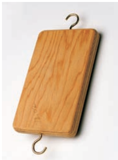
Photo 1 —Above, Typical MEE test blank. MEE blanks are dried out in the Arizona room and, after coating, saturated in the Florida room.
