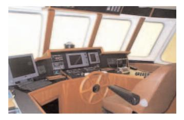
The wheelhouse is located well aft on the main deck to maximize the comfort level of the crew whilst at sea. The saloon is located two steps down to reduce the vertical centre of gravity, and to enhance the stability. The owners did not request a flybridge, although one could easily be added if required.
